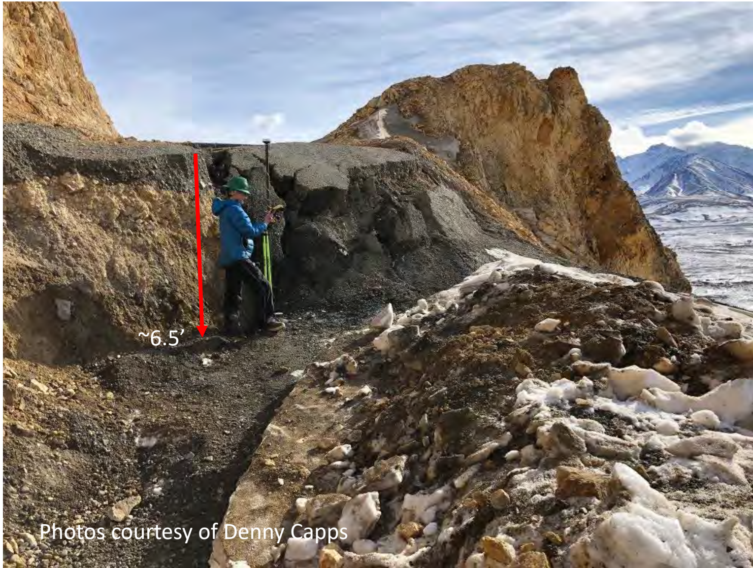
Figure 9. Site Photo from March 21, 2019. Rate of Movement from Surface Measurements: ~0.4 inches/day or ~12 inches/month
