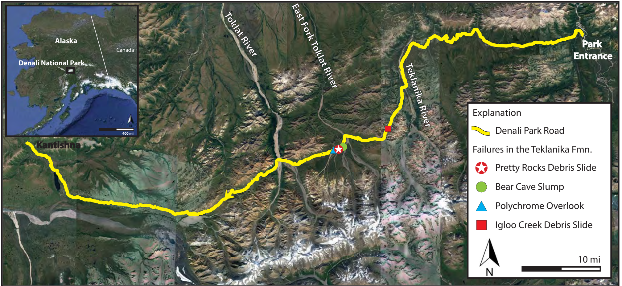
Figure 1: Map of Denali Park Road highlighting failures that have occurred or are occurring within the Teklanika Formation. Note that 3 of the 4 failures are occurring in close proximity to one another within Polychrome Pass. Imagery from Google Earth.
