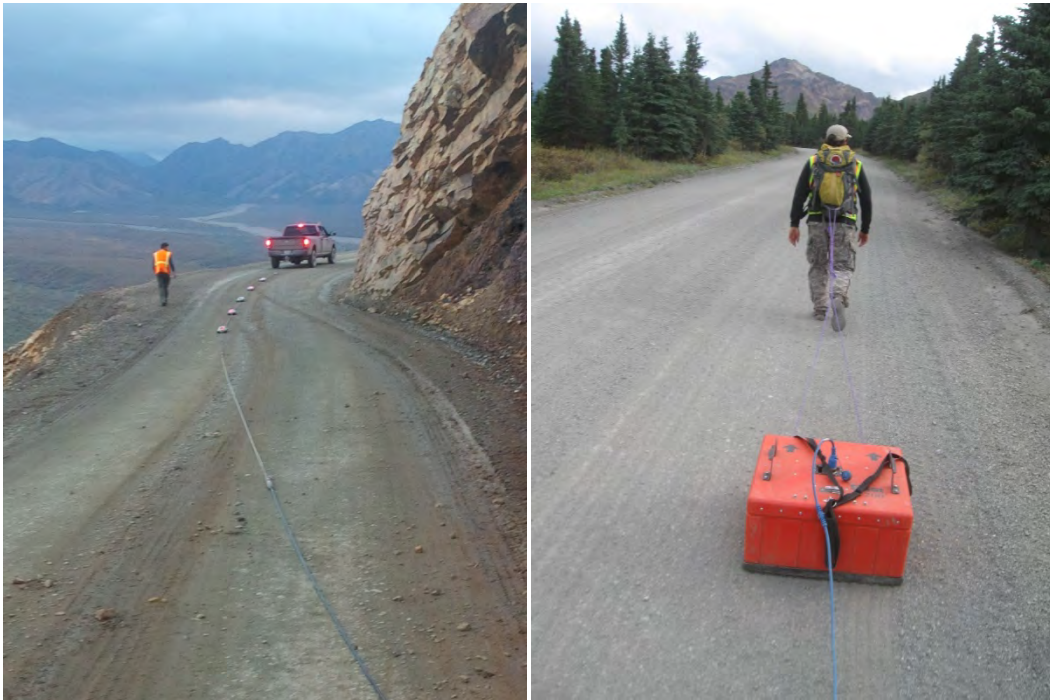
Figure 7. CCR Survey and GPR Survey. The CCR array (left) is being pulled by truck along the Polychrome Pass section, August 25, 2016. The 200MHz GPR (right) is pulled manually along the Igloo Forest Section, August 24, 2016.
