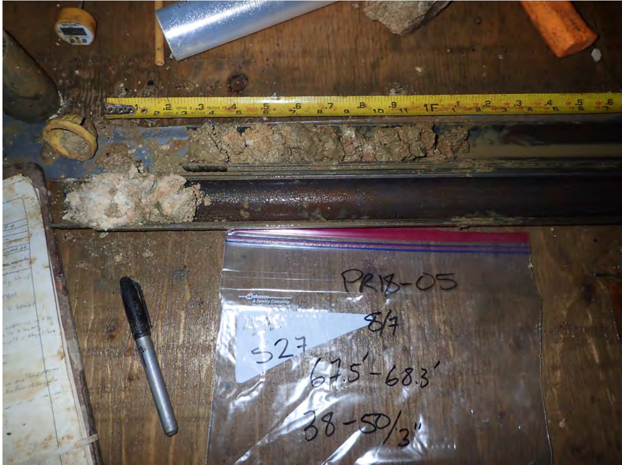
Figure 24. Slope inclinometer measurements in PR18-05 and a photograph of the core recovered that contains the abrupt failure plane and change in materials.
