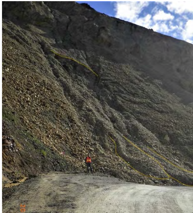
Figure 24: Debris flows seen looking northeast. Scarp and lobe deposits highlighted for clarity. Eastern lobe extends beyond the photo frame.
