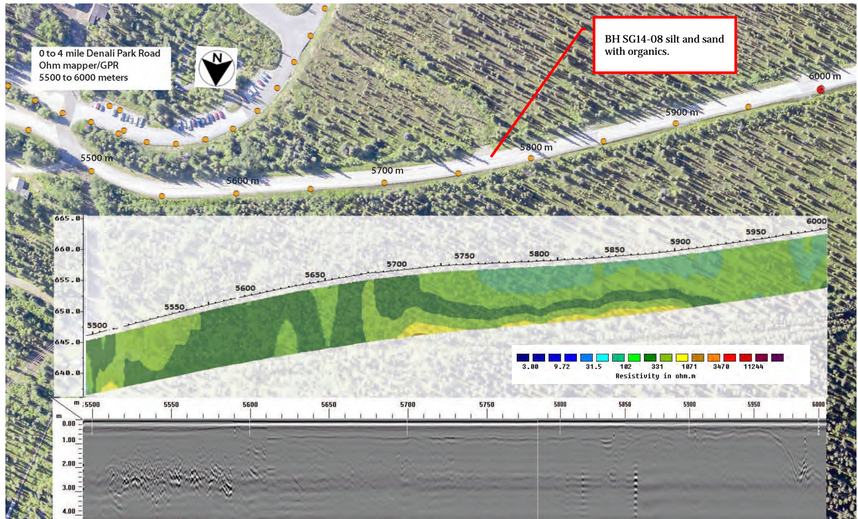
Figure 19. Park Road mile 0 to 4, 5500m to 6000m (18044-ft to 19685-ft). Very low ohm-m values which started at 5450m in the previous section continue through this section as well. An increase in near surface moisture content is inferred starting at 5750m though to 6000m. Moderate ohm-m values are noted from 5700m to 5900m and this may be a rising bedrock surface or possibly ice-moderate to ice-rich permafrost at depth. The GPR returns are very minimal through this section indicating increase in moisture content or clay mineral composition. TH83-5 drilled in this vicinity showed peat and silty fine sand, unfrozen (Fig. 72).
