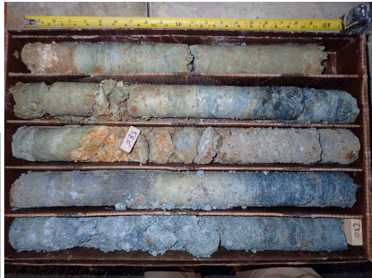
Figure 22. Photographs of the cored materials during the drilling operations. The lower left is primarily mafic (basalt) intrusion rock and the right is very weak rhyolite grading to rhyolitic volcanic ash tuff from top to bottom.
