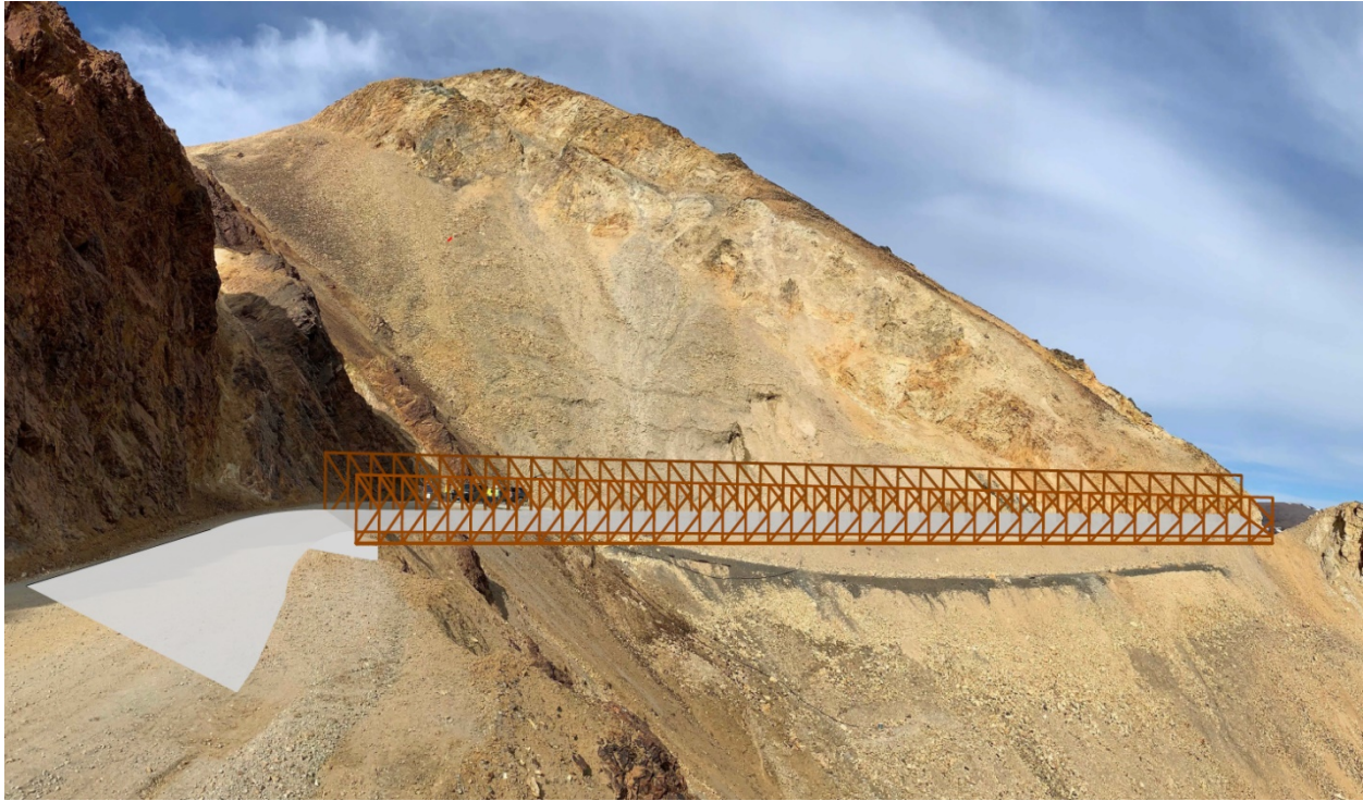
Figure 10. Rough concept of a Modular Steel Truss constructed at Pretty Rocks Landslide
