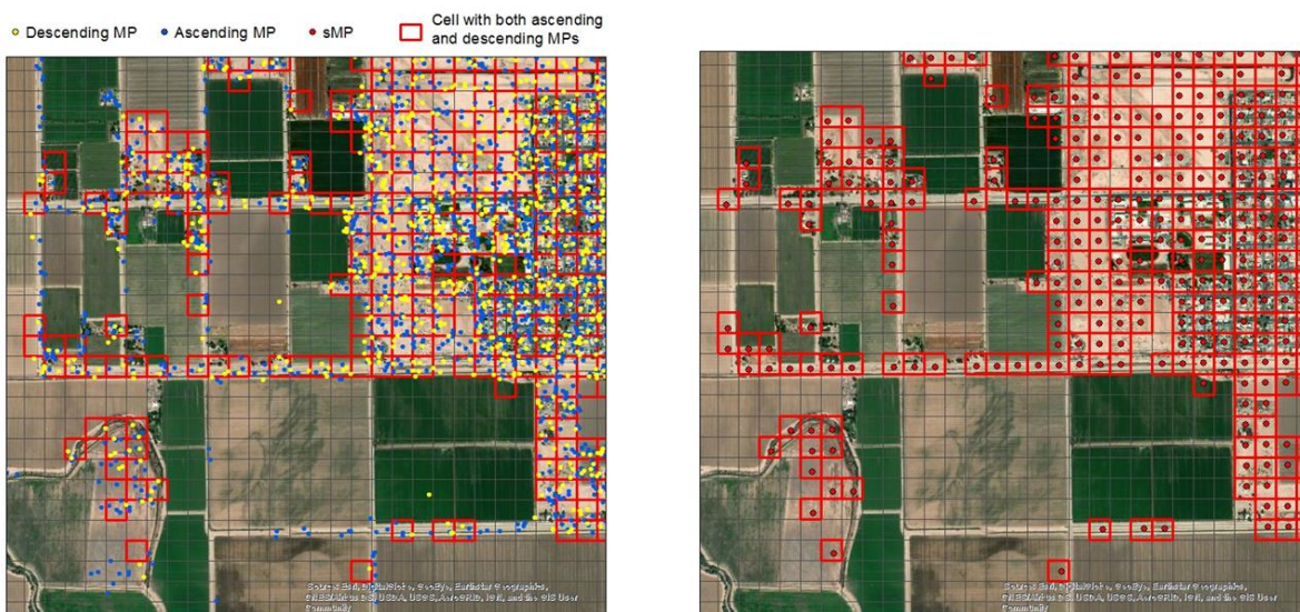
Figure 11: 2-D measurements are estimated by subsampling ascending and descending data on a common spatial grid. The measurements of all MPs contained within the same cell are averaged to produce 2-D measurement points located at the centre of the cell. The 2-D procedure only produces readings for cells containing MP from both orbits (red cells).
