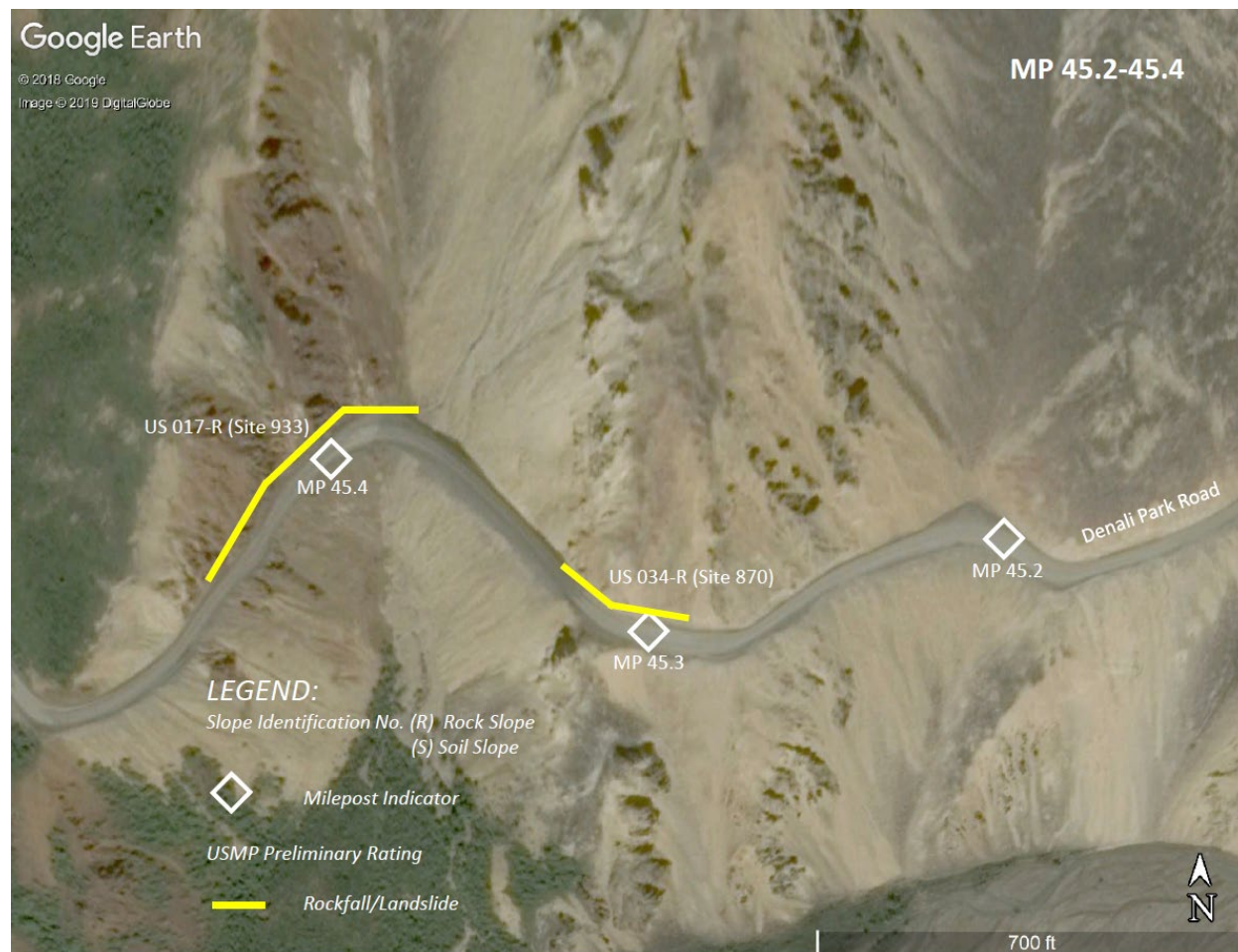
Figure 5-25. Overview of sites 870 and 933 between MP 45.17 and MP 45.32 on the Denali Park Road in Alaska (U.S Department of Transportation, December 2019).
