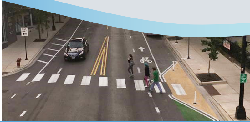
Figure 1. Graphic. Example of dashed bike lane on Milwaukee Avenue. Dashed bike lane positions motorists closer to the center line and provides more space for people on bikes.
