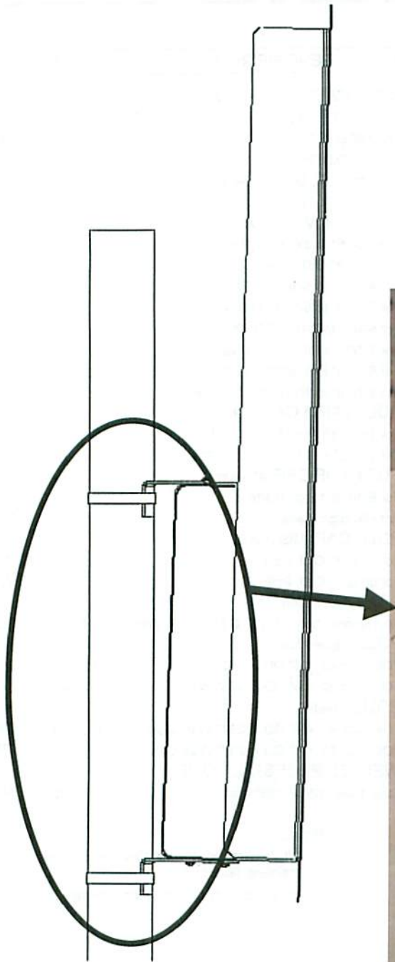
VSC-1820 Pole Mounting View with Strapping; U-Bolts mounting is similar Dimensions and material shown on Page 1
