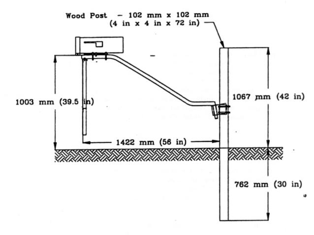
Figure 1. Schematic of Roadside Safety Devices Swing-Away Mailbox Support Design.
