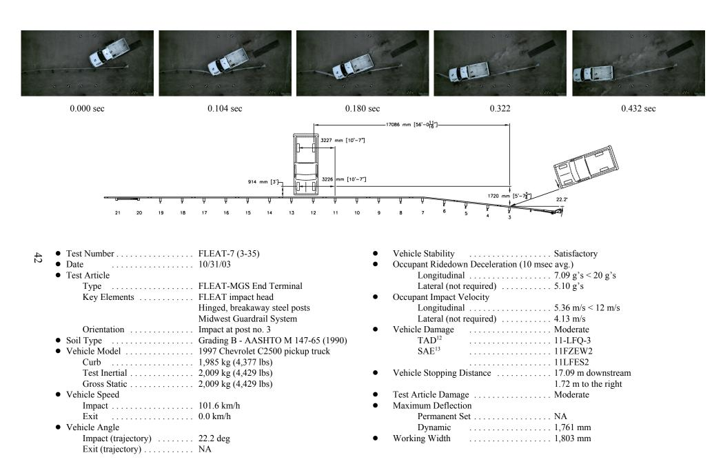
Figure 24. Summary of Test Results and Sequential Photographs, Test FLEAT-7
