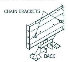
QUADGUARD UNIVERSAL DIAPHRAGM WITH MODIFIED CARTRIDGE CENTERING/BAY CHAIN BRACKETS
