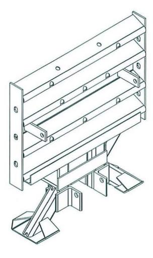
QUADGUARD® MODIFIED DIAPHRAGM WITH ELITE FEATURE MOUNTING HOLES
