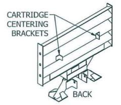
QUADGUARD ELITE DIAPHRAGM WITH EXISTING BAY CHAIN BRACKETS
