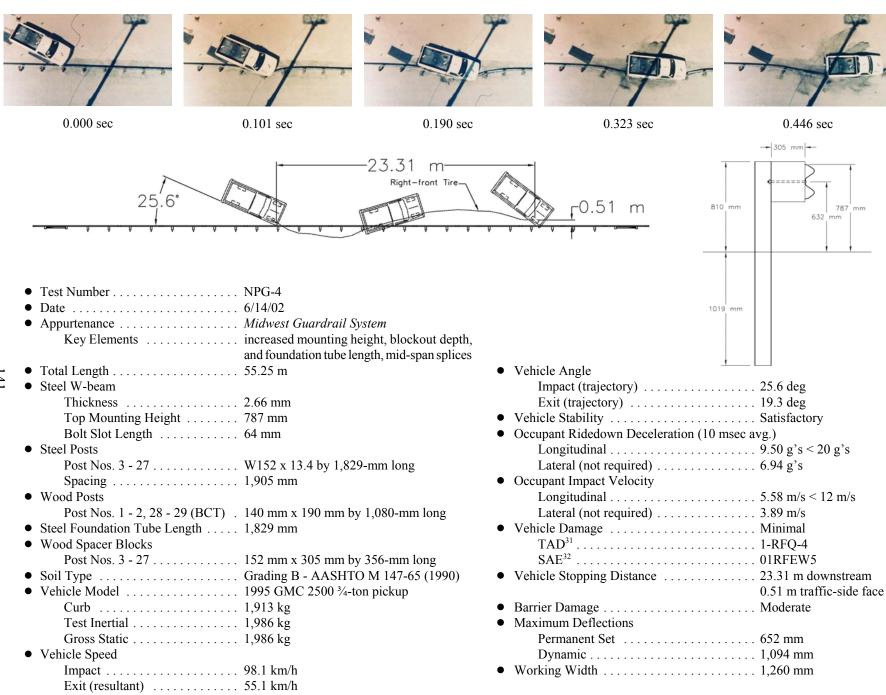
Figure 87. Summary of Test Results and Sequential Photographs, Test NPG-4
