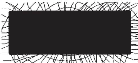
Case 3: Significant overall damage. Driver cannot readily see ahead to navigate to a safe stop.
