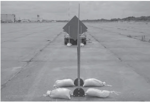
Figure 7.15. Pivoting dual-upright system used in Test 6.
