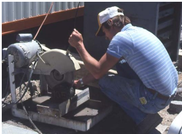
Exhibit 4-34 Sawing to Separate Pavement Layers
