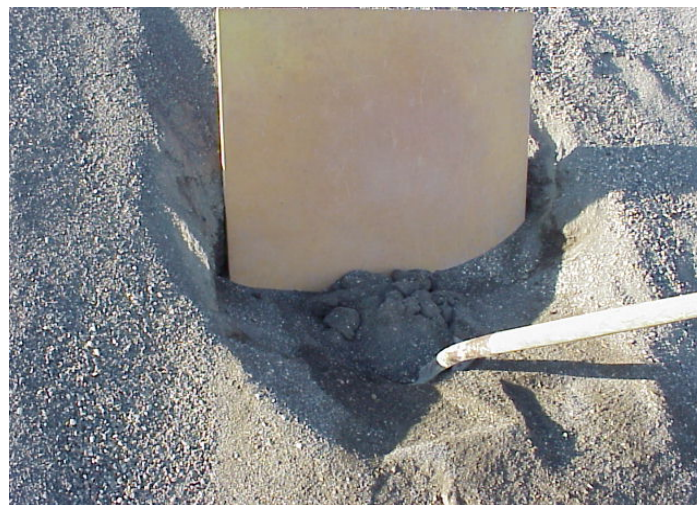
Exhibit 3-14 Proper Use of Shield for Sampling
