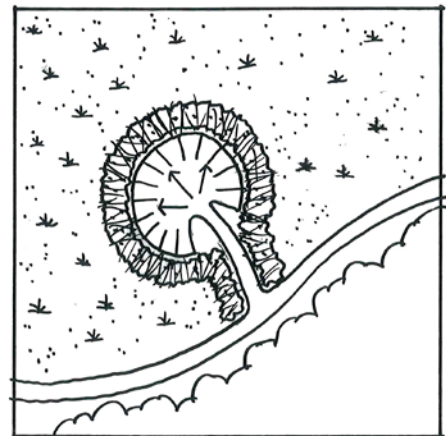
NDS features receive, clean and detain or retain runoff from roadways and other impervious surfaces; they can buffer habitat areas from negative ecological impacts.
