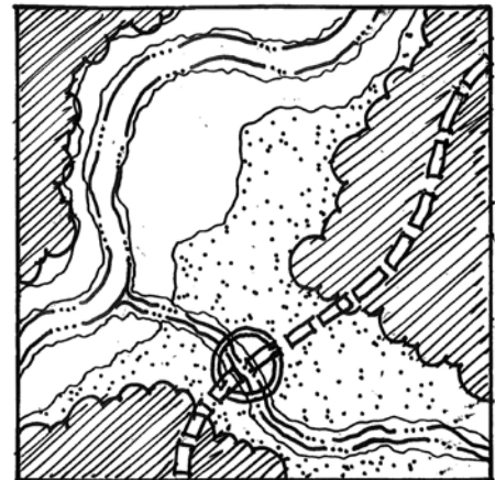
Examine the roadway corridor for locations where organisms would prefer to cross in the absence of a roadway. Study topography, vegetation patterns and hydrology along the corridor.
