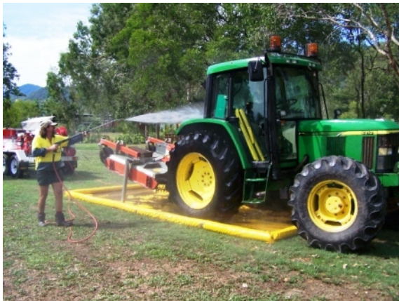
Figure 20: Secondary containment for maintenance and fueling and clean-up operations
