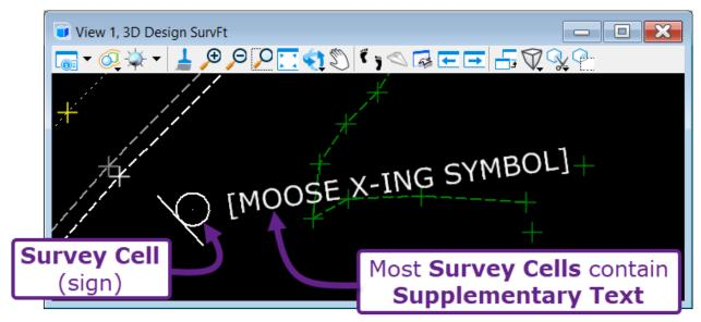
**PROCESS 3 – Creating the Existing Ground Terrain Model:** Ground Points and select Existing Linework elements form the Existing Ground Terrain Model.
