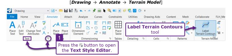
**IMPORTANT:** Before using this tool, a custom **Text Style** and **Dimension Style** must be created. The FLH WorkSpace does NOT contain **Text/Dimension Styles** that are appropriate for contour labels.
