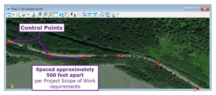
Survey Points are Collected: The field personnel work down the length of the project to collect Survey Points. When a Survey Point is collected, it is assigned a Point Code that consists of a 3-digit type identifier and a 2-digit line identifier.
