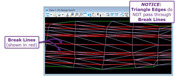
**Break Lines** are necessary to capture abrupt changes in slope and deflections in a surface (i.e., a sharp ridge). If Break Lines are NOT used, then the Terrain Model may interpolate through important deflection areas.
