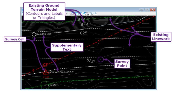
**The Existing Ground Terrain Model:** The Existing Ground Terrain Model is a 3-dimensional digital surface that characterizes the existing ground elevations in the project area.
