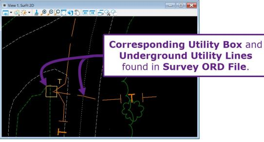
**Examine Existing Linework for Discrepancies:** Ensure that Existing Linework is joined together or segmented appropriately.
