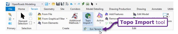
**NOTE\*:** This tool is powered by the ESRI World Elevation map. The source and accuracy of the imported Terrain Model depends on the selected area. Before using this tool, the ESRI World Elevation map can be accessed through the following website:
