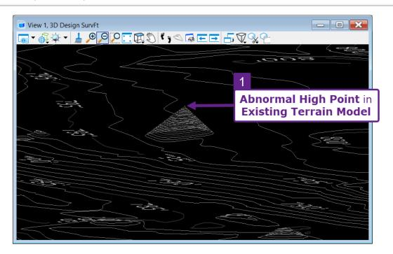
Elevation busts are more likely to happen in the vicinity of culverts, bridges, and other complex areas. Examine these complex areas for faulty elevations points. In the example shown below, a Bridge Deck Point shot is included in the Existing Ground Terrain Model. Bridge points do NOT represent the Existing Ground elevation and should NOT be included in the Terrain Model.
