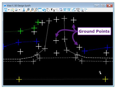
Survey Cells: Signs, Trees, and Utility Features: In processing, Survey Cells are automatically placed at the point locations of non-linear features (i.e., signs, trees, and utility features). Each non-linear point code has a corresponding Survey Cell graphic. For example, the point code for a sign is 232. When a point with the 232 code is imported into ORD, the sign Survey Cell is automatically placed at the point location.
