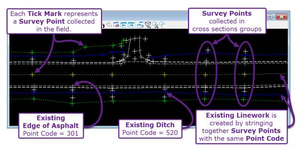
For roadway projects, the field personnel typically collect Survey Points in cross section groups. Typically, cross section groups span the entire width of the existing road embankment. For example, the cross section group might begin at the top of cut, and then move consecutively to the ditch line, edge of shoulder, edge of asphalt, centerline of road, and so on. If necessary, important features outside of the existing road embankment may also be collected in the cross section group.
