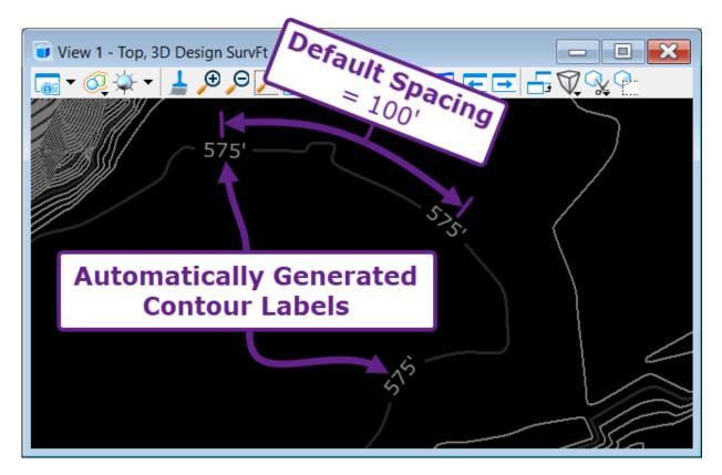
**TIP:** Contour Labels can be created and placed at a fixed location with the *Label Terrain Contours* tool. See **5B.7 Label Terrain Contours tool**.
