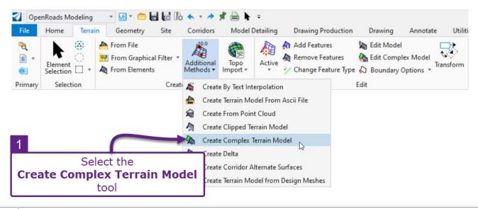
From the Ribbon, select the *Create Complex Terrain Model* tool: [**OpenRoads Modeling**  $\rightarrow$  **Terrain**  $\rightarrow$  **Create**  $\rightarrow$  **Additional Methods**]. **IMPORTANT:** The Imported Terrain Model must be set as the **Primary**. The Existing Ground Terrain Model must be set to **Merge**. This configuration is necessary to ignore the Imported Terrain Model in areas of overlap with the Existing Ground Terrain Model.
