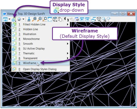
Changing the Display Style to an **Illustration** style will show the triangles as solid mesh. The edges of the triangles are shown.
