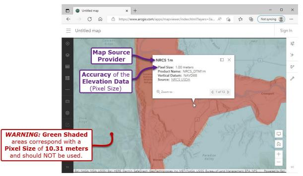
The **Pixel Size** corresponds with the accuracy of the elevation data in the area.
