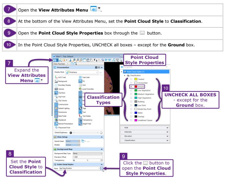
With ONLY the Ground points displayed, the Terrain Model can be created. The *Create From Point Cloud* tool is used to convert the Point Cloud into a Terrain Model.
