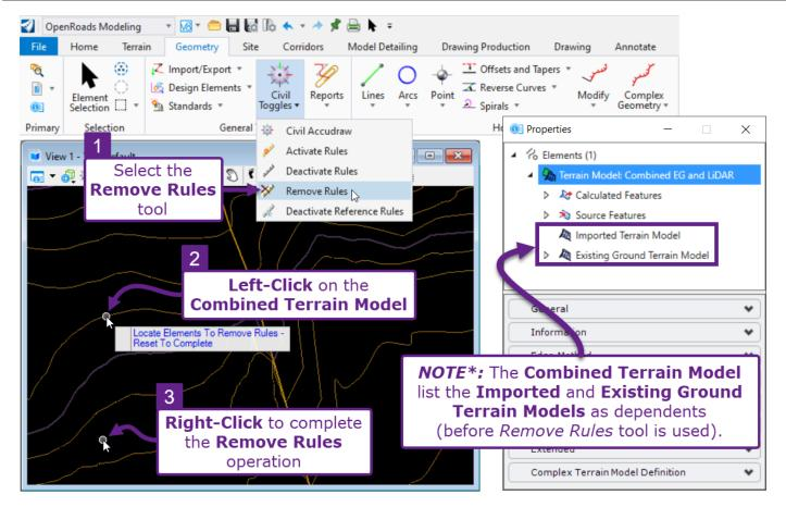
To delete the Imported and Existing Ground Terrain Models, open the **Explorer** and open the **OpenRoads Model** drop-down. Locate the Terrain Models to delete under the **Terrain Models** drop-down.
