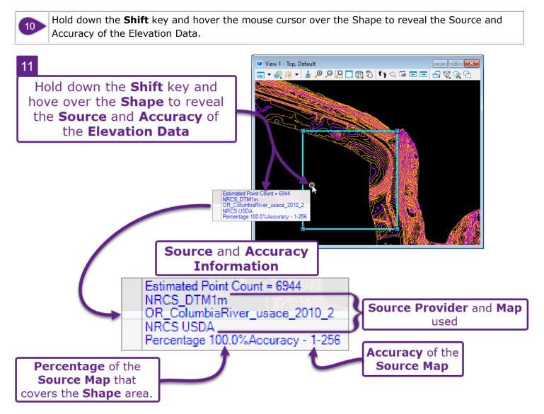
**Source Provider and Map:** This information designates the providing agency and map used for the elevation data.
