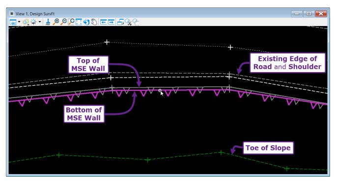
Shown below on the left is how the Terrain Model would look if NO Break Lines were used. In this case, the Terrain Model is created from Survey Points ONLY. As shown in the Profile view, the abrupt change from the MSE wall is NOT captured.
