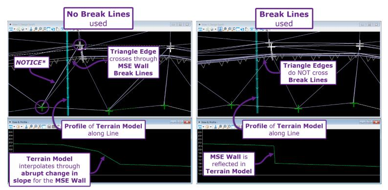
Shown above on the right is how the Terrain Model looks when Break Lines are used to control triangulation. In this case, the Triangle Edges NEVER cross through the Top and Bottom of MSE Wall Break Lines. The abrupt changes in slope that the Break Lines correspond to are reflected in the Terrain Model.
