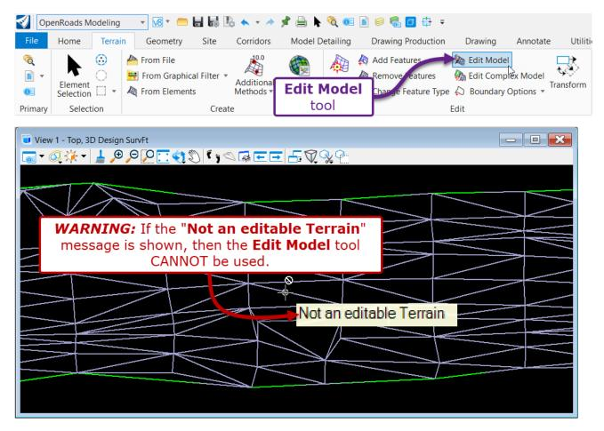
*Rules* dynamically link a Terrain Model to the graphical elements that were used to create it. If a graphical element is manipulated, then the Terrain Model will automatically update due to the *rule* relationship.
