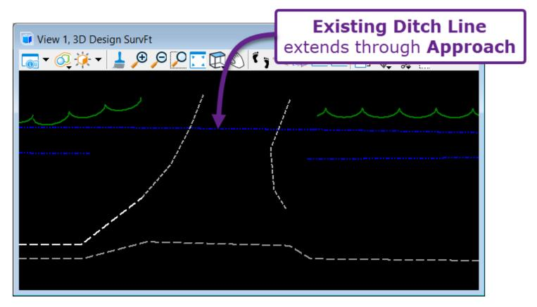
Also, ensure that Existing Linework reflects the correct feature. As an example, the line on the bottom is depicted and set to the Jersey Barrier level; but this feature is a guardrail in the field.
