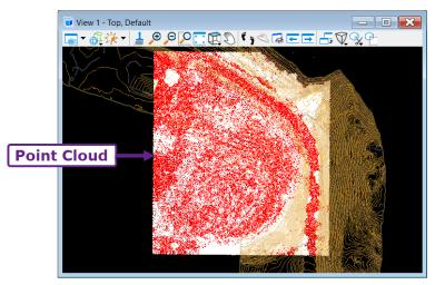
All points that DON'T represent the Ground must be toggled OFF before creating a Terrain Model. Through the **Point Cloud Style Properties** box, points can be toggled OFF by Classification:
