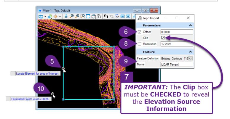
After step (10), the source provider and accuracy of the elevation data is shown in the Floating Dialogue Box.
