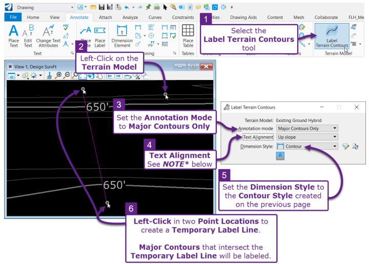
**NOTE\*:** There are two **Text Alignment** (step 4) settings: "Up Slope" and "Follow Line". This setting affects the orientation of the contour labels. The User may need to experiment with both settings to show the label right-side up. In the graphic above, the Text Alignment is set to "Up Slope" and both labels are shown correctly. In the graphic below, the Text Alignment is set to "Follow Line" and the top label is shown upside-down.
