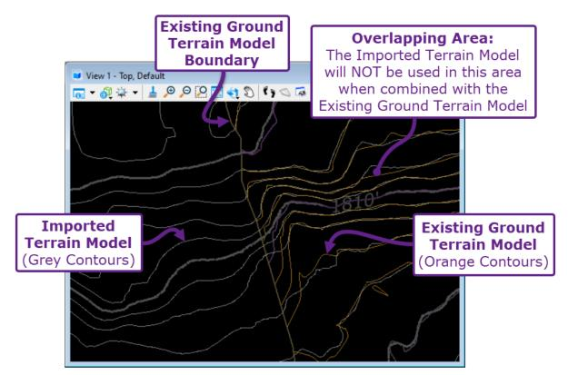
Combining Terrain Models is performed with the *Create Complex Terrain Model* tool. This tool is discussed in greater detail in <u>22E – Merge Terrain Models</u>.
