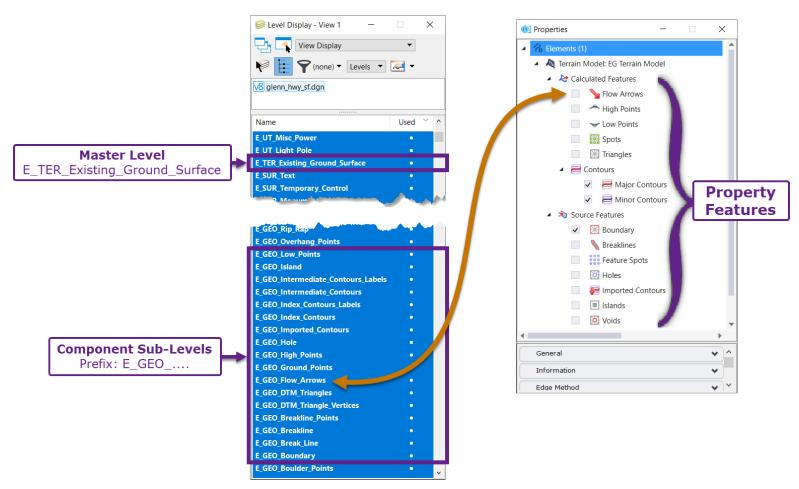
For example, the display of the Boundary element can be toggled OFF with the "E\_GEO\_Boundary" Level.
