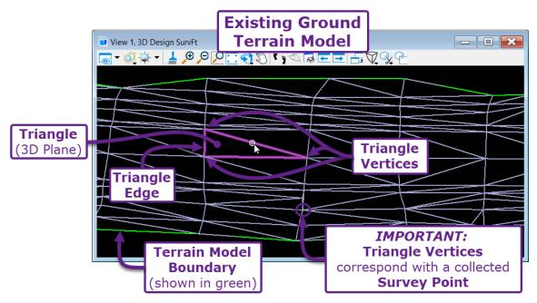
The term **Triangulation** refers to the configuration and layout of triangles in a Terrain Model.
