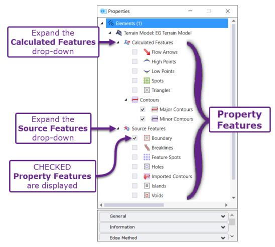
**Calculated Features:** Calculated Features are automatically generated by the Terrain Model. For example, Contours are calculated through interpolation based on the Break Lines and Ground Points elevations used to create the Terrain Model.
