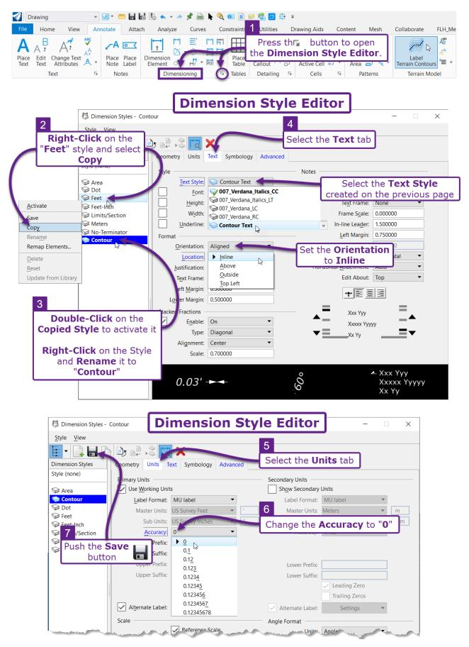
After creating the contour label **Text** and **Dimension Styles**, the *Label Terrain Contour* tool can be used. In step 5, select the contour label style created on the previous page.
