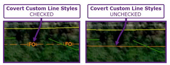
**Built-In** Styles may appear dashed or dotted in ORD but will ALWAYS be shown as solid lines in Google Earth. For example, Cut and Fill Lines are assigned to Built-in Style (1) and Built-in Style (3), respectively. As a result, Cut and Fill Lines are shown as solid lines in Google Earth.
