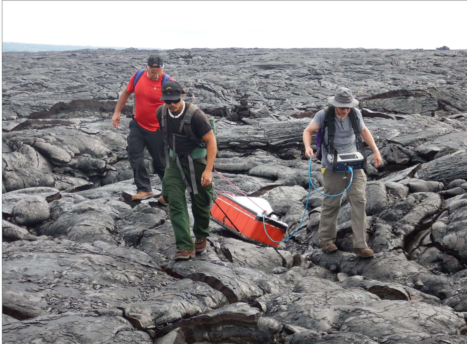
When Kilauea Volcano erupted in 2014, the lava flow began advancing towards the community of Pahoa. Geophysical techniques and testing were used in advance of the emergency construction, to identify lava tubes and hot spots that mitigated risk of delay or injury and supported construction necessary to maintain evacuation routes.
