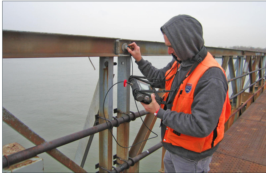
Ultrasonic Testing of Truss Pin
