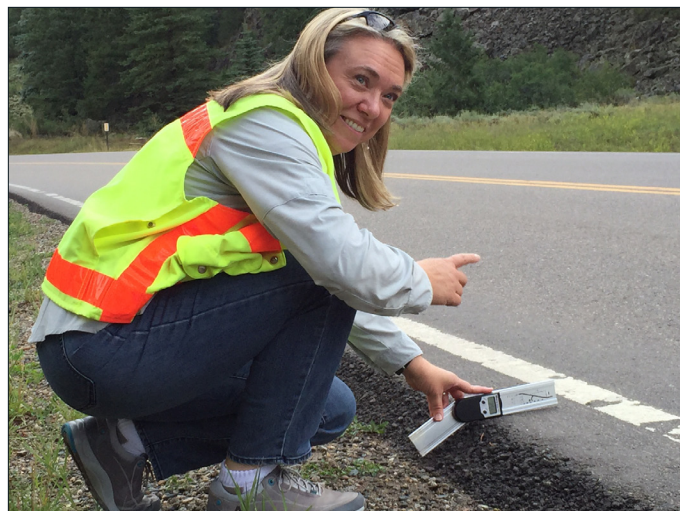
Highway Safety Engineer Measuring Pavement Edge Slope
