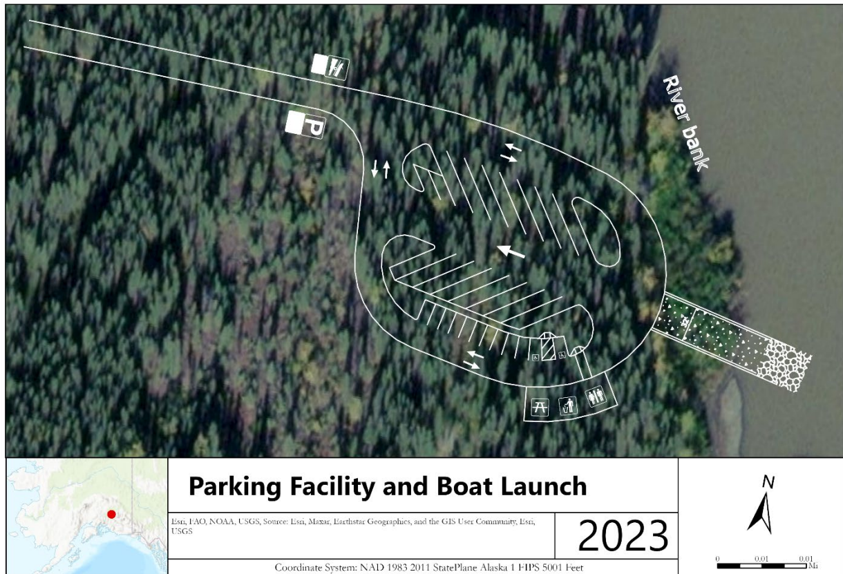
Figure 6. Conceptual design of parking lot and boat launch with existing imagery.
