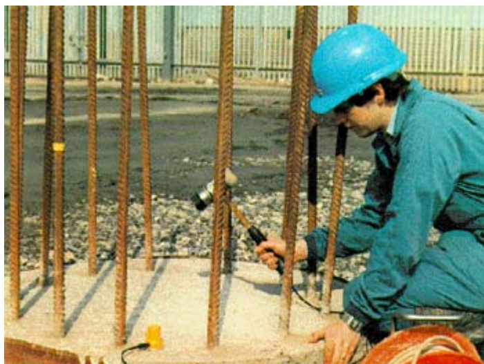
FIGURE 20. Low-strain impact test with instrumented hammer and geophone sensor.
