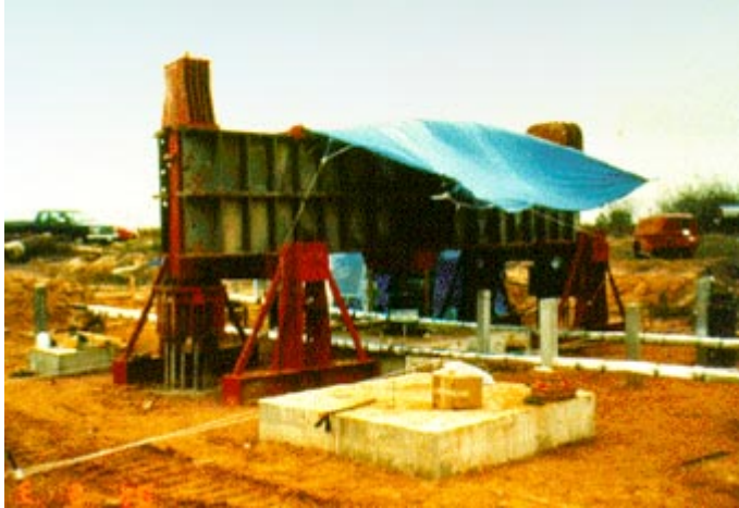
FIGURE 22. Load testing of large model spread footing.
