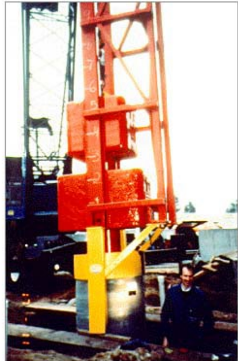
Figure 26. FIGURE 26. Large-strain dynamic load testing using drop hammer.
