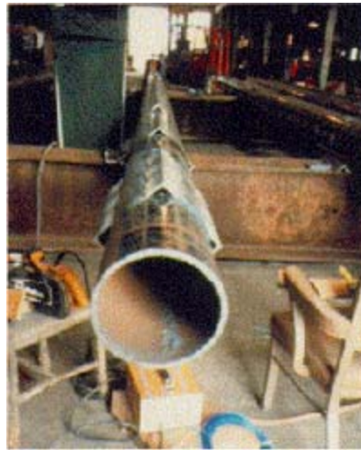
FIGURE 4. Field instrumentation of a pipe pile for field load test in sand.
