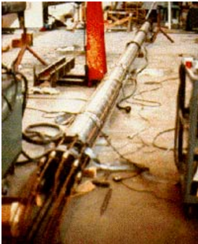
FIGURE 3. Lab instrumentation of a pipe pile for field load testing in clay.
