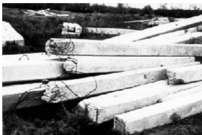
FIGURE 5. Concrete piles damaged by difficult driving conditions.
