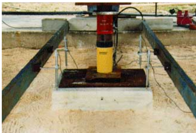
FIGURE 28. Spread footing load test on reinforced soil foundation.
