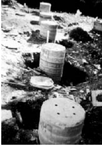
FIGURE 17. Drilled shafts with and without defects.
