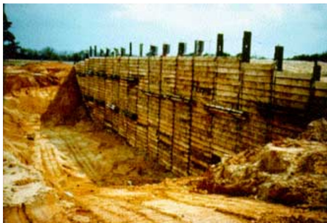
FIGURE 32. Full-scale ground anchor test wall at TAMU NGES.
