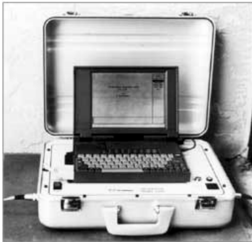
Figure 30. Polarization Resistance (PR) monitor for corrosion potential.
