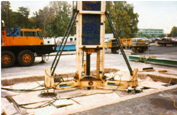
FIGURE 24. Vertical statnamic load test on model pile group at TFHRC.
