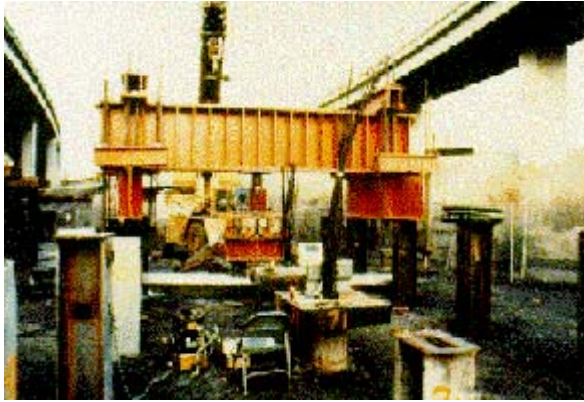
FIGURE 10. Load testing of micropiles in California.
