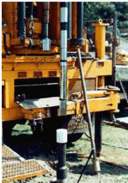
Figure 45. Torsional impulse shear test to obtain earthquake engineering soil parameters at Treasure Island.
