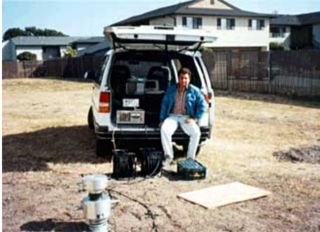
FIGURE 46. Controlled source spectral analysis of surface waves (CSSASW) testing at Treasure Island.
