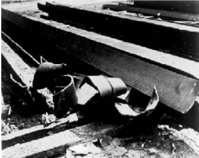
FIGURE 6. Steel H-piles badly damaged by hard driving.
