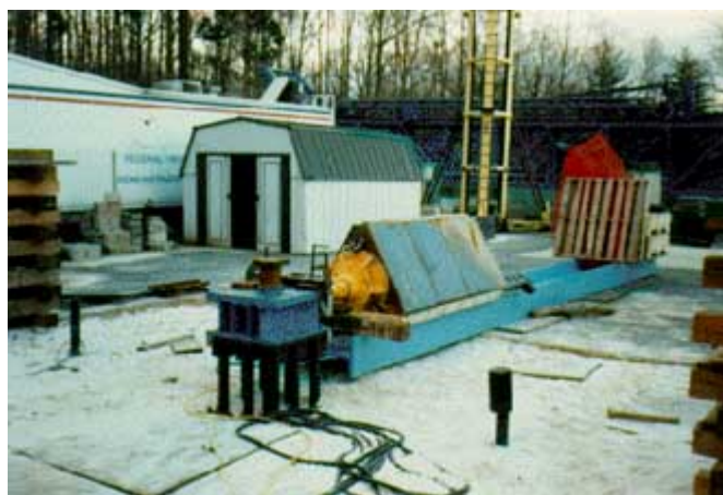
FIGURE 50. Lateral statnamic load test on model pile group at TFHRC.
