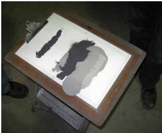
Fly ash with different carbon content levels. Source: FHWA.
