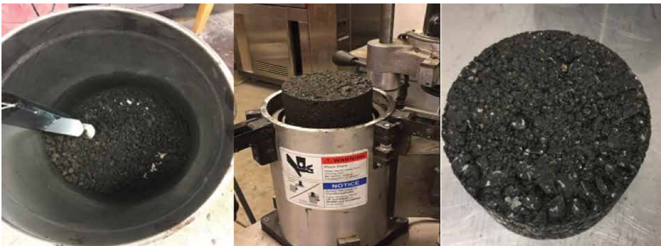
Researchers created a rotary reactor to simulate the production of the hot-mix bio-binder through mixing aggregates with bioasphalt. © 2017 Department of Civil and Environmental Engineering, Washington State University.
