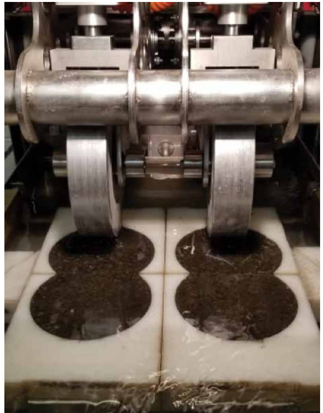
The Hamburg wheel tracking test is conducted on a hot-mix bio-binder to evaluate any permanent deformation. © 2017 Department of Civil and Environmental Engineering, Washington State University.
