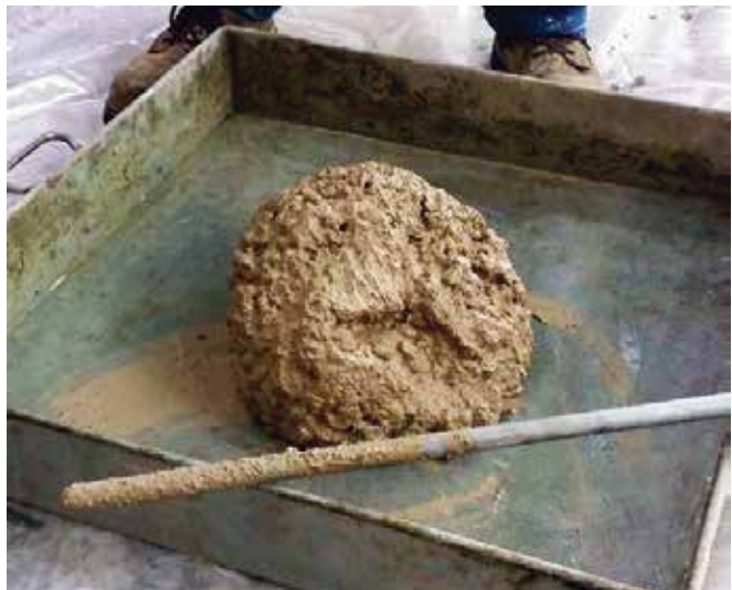
Concrete slump made of an alternative cementitious material (calcium sulfoaluminate). © College of Engineering, Georgia Institute of Technology.
