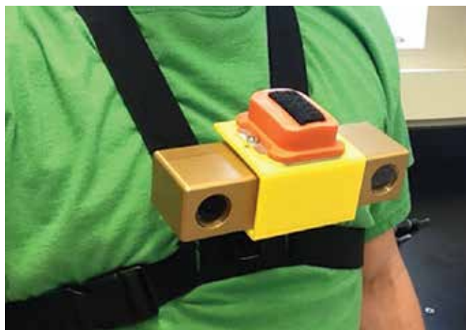
A chest-mounted stereo camera and inertial measurement unit form part of a pedestrian navigation system developed by Auburn University. © Auburn University.
