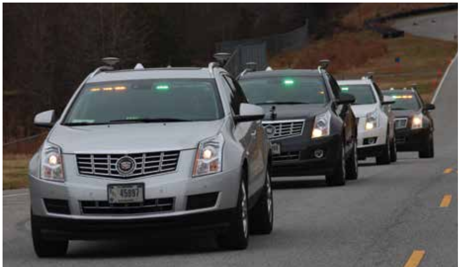
FHWA test vehicles simulate a “platoon” of vehicles using cooperative adaptive cruise control. Source: FHWA.
