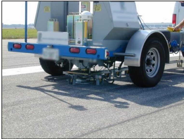
Figure 4. Photo. Impulse loading or FWD device.
