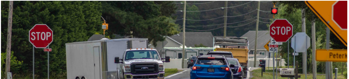
Stop Sign with ALL WAY plaque and flashing beacons. Photo courtesy of Rummel, Klepper & Kahl, LLP (RK&K).
