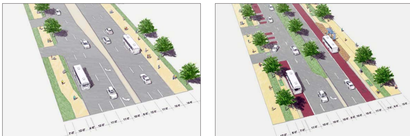
Figure 1. Illustration. Existing configuration (left) and vision (right) for changes to East Arapahoe Avenue, including bus rapid transit lanes and separated bike lanes.
