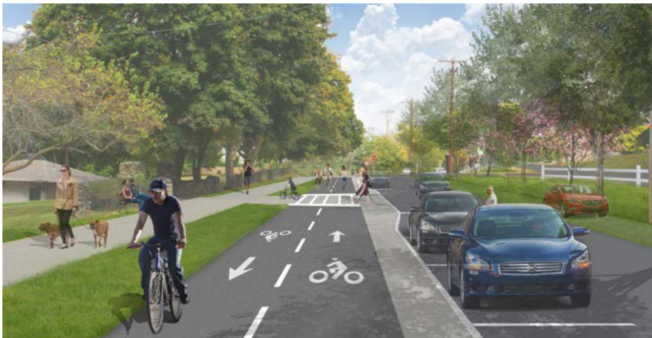
Figure 4. Image. Rendering of proposed changes to Commonwealth Avenue with new sidewalk and two-way separated bike lanes.
