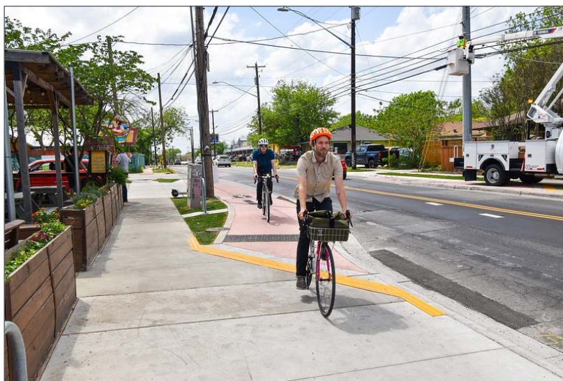
Figure 4. Image. Separated bike lane to sidewalk transition that separates users in space in Austin.
