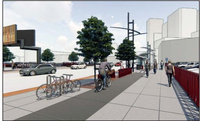
Figure 3. Illustrative rendering for Hennepin Avenue redesign showing separated, behind-the-curb bike lane, widened sidewalk and transit stop.
