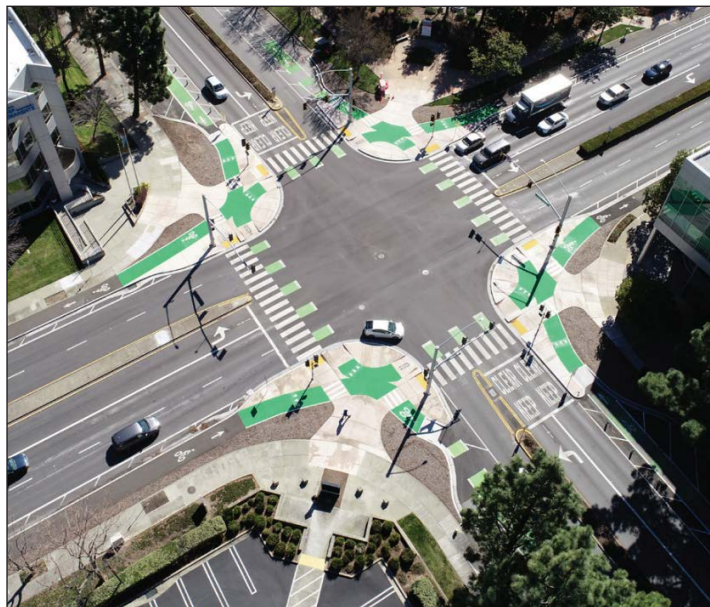
Figure 1. Image. Protected Intersection in Fremont, CA, at Civic Center Drive and Walnut Avenue.
