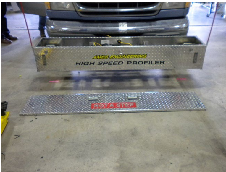
Figure 11. Photo. High-speed line laser. Source: CSTI
