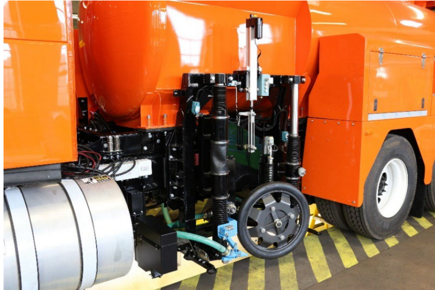
Figure 7. Photo. Example of SFC: Sideway-force Coefficient Routine Investigation Machine (SCRIM). Source: CSTI
