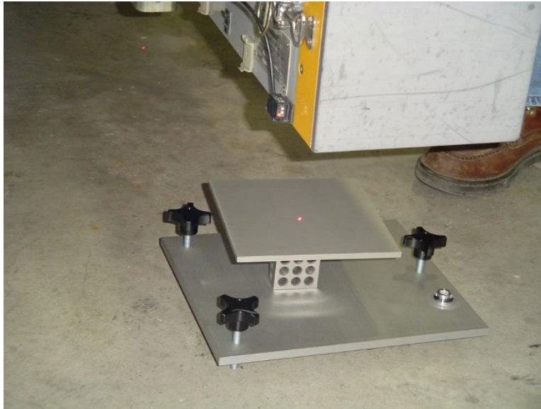
Figure 10. Photo. High-speed single spot laser. Source: CSTI
