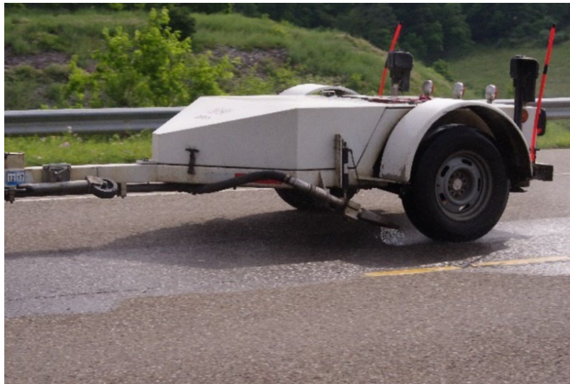
Figure 6. Photo. Example of LFC: 100% slip-LWST. Source: CSTI
