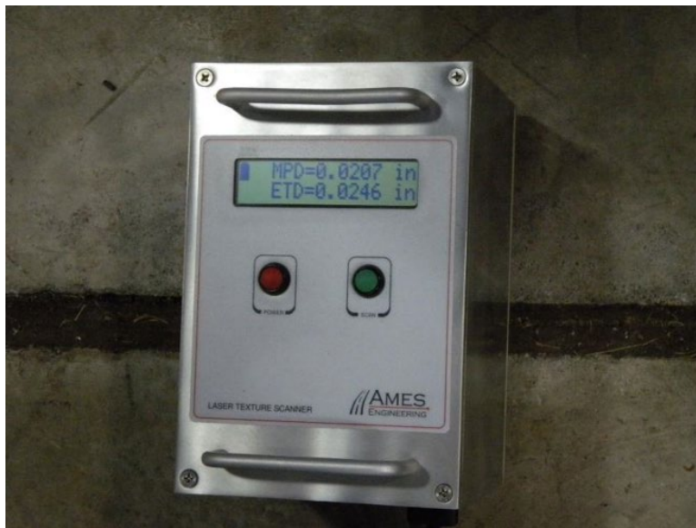
Figure 9. Photo. Static line laser: Texture Analyzer. Source: CSTI
