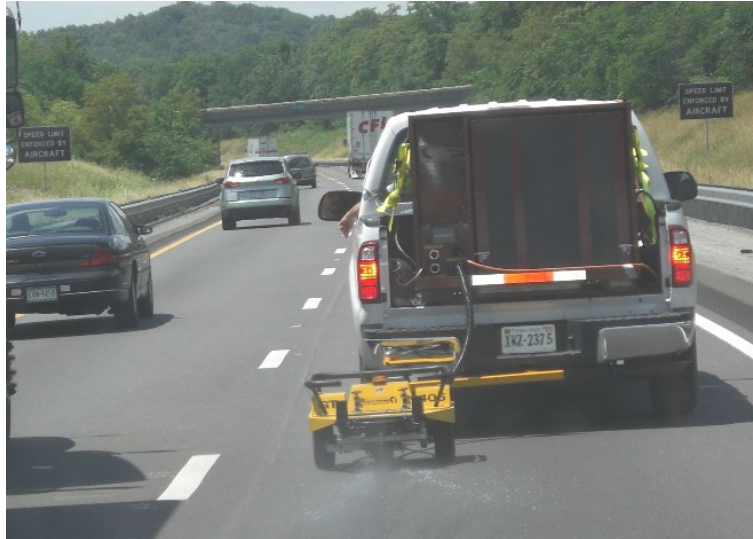
Figure 5. Photo. Example of LFC: Fixed slip device-grip tester. Source: CSTI
