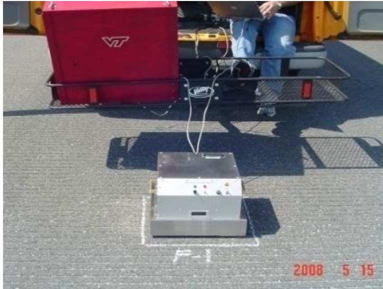
Figure 8. Photo. Static single spot laser: Circular Track Meter. Source: CSTI
