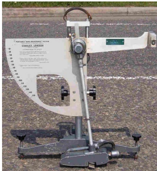
Figure 4. Photo. Example of a slider: British Pendulum Tester. Source: CSTI
