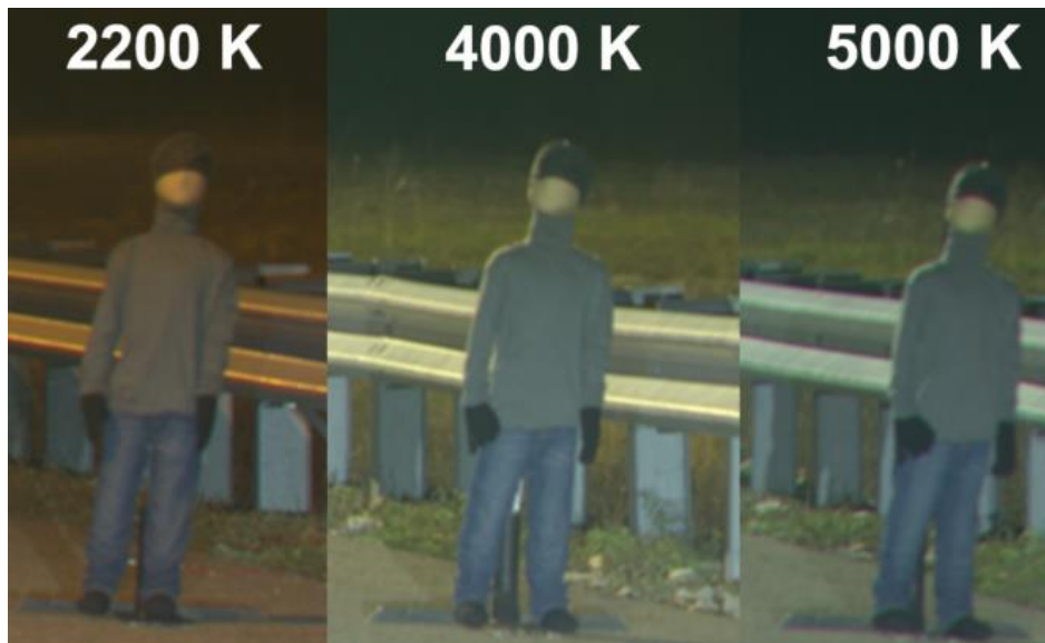
Figure 19. View of child-sized mannequin under each SPD
