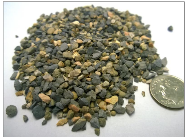
FIGURE 6 – Calcined Bauxite Crushed & Graded.
