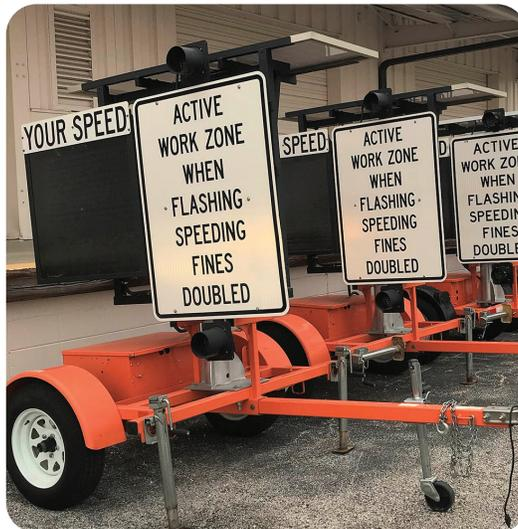
AWAD installed on portable trailers ready for deployment to work zones. Photo courtesy FDOT.
