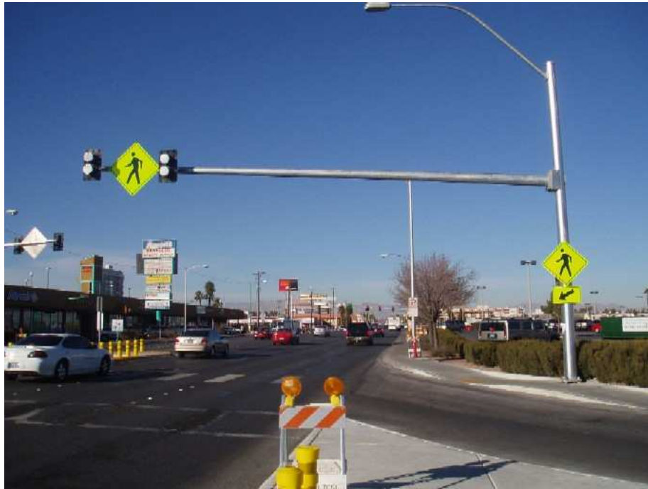
Figure 9: Pedestrian Activated Flashing Yellow
