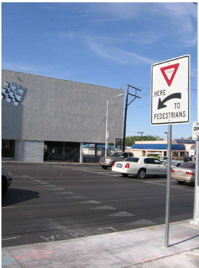
Figure 48: “Advanced Yield Markings” installed at Site 19
