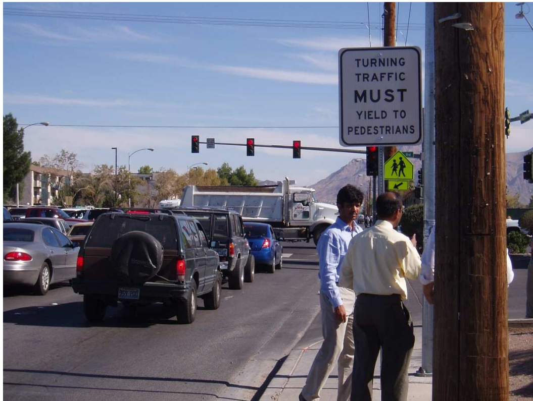
Figure 40: “Turning Traffic Must Yield to Pedestrian” signs installed at Lake Mead Boulevard and Pecos Road
