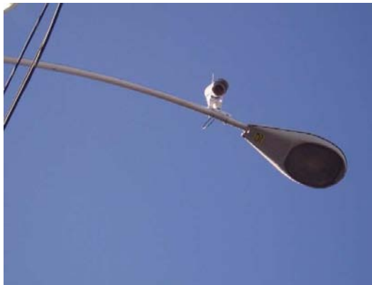
Figure 50: Automatic Pedestrian Detection
