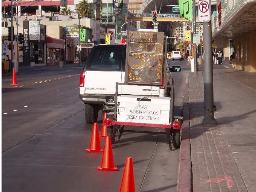
Figure 43: Portable Speed Trailer on Fremont Street
