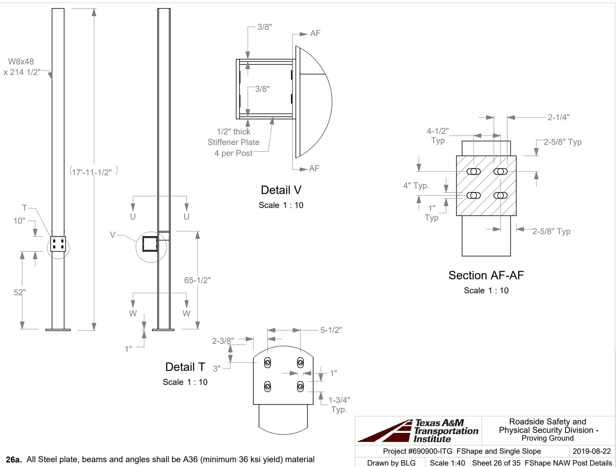
26a. All Steel plate, beams and angles shall be A36 (minimum 36 ksi yield) material
