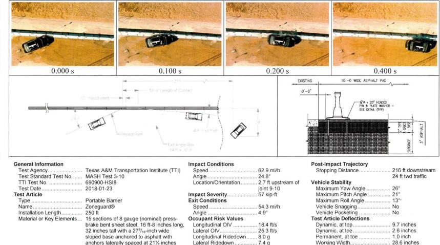
Figure 5.6. Summary of Results for MASH Test 3-10 on Zoneguard® Barrier.
