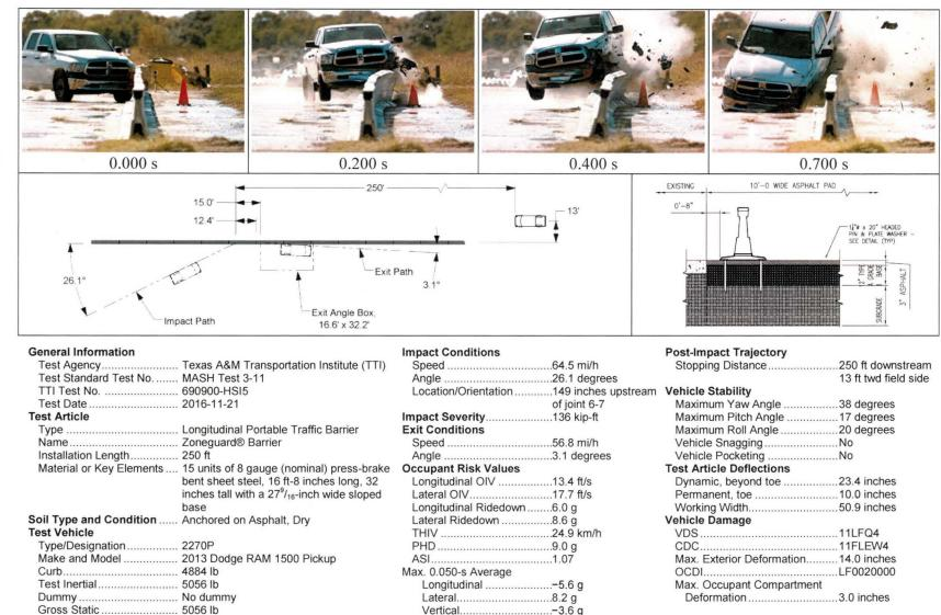
Figure 5.6. Summary of Results for *MASH* Test 3-11 on Zoneguard® Barrier Anchored with Round Headed Anchoring Pins at 33 ft-4 inch Spacing, on center, on Asphalt Pavement.
