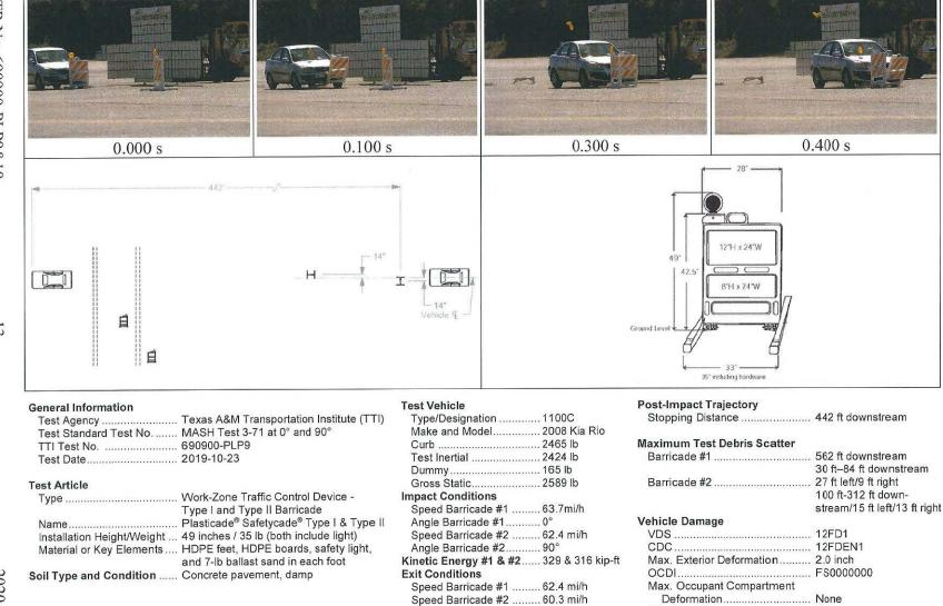
Figure 5.7. Summary of Results for MASH Test 3-71 at 0° and 90° on Safetycade® Type I and Type II Barricades
