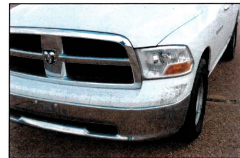
Damage to vehicle after Test Nos. 690900-DTC19-1 through 4.
