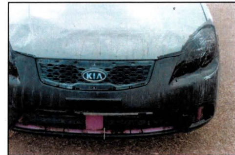
Damage to vehicle after Test Nos. 690900-DTC19-5 through 8.
