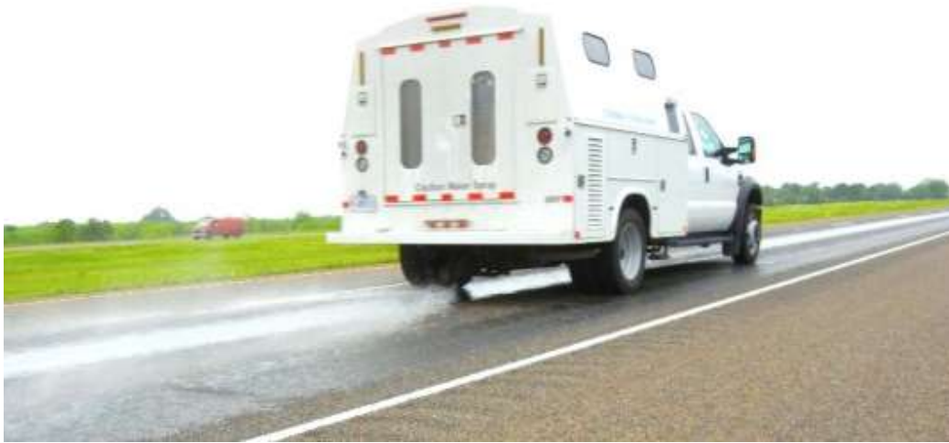
Figure 2.3 A Dynatest 6875H highway friction tester that maps friction continuously along a pavement section. (From http://www.thetranstecgroup.com/fhwa-providing-friction-tester-demonstrations/ )
