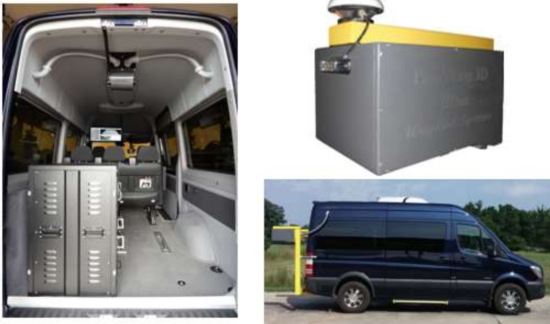
Figure 2.1. A PaveVision3D Ultra data collection vehicle used for the research
