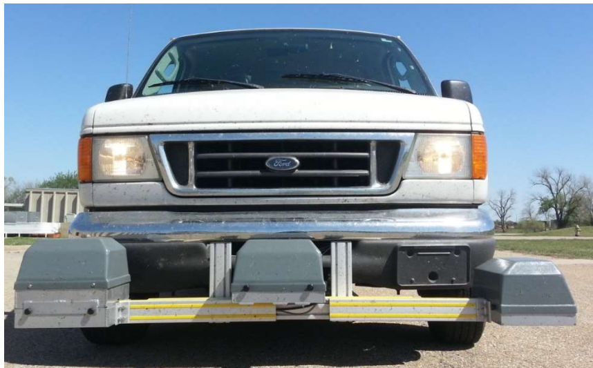
Figure 2.2 AMES 8300 high speed profiler used to collect Macro Surface Texture data and profile data
