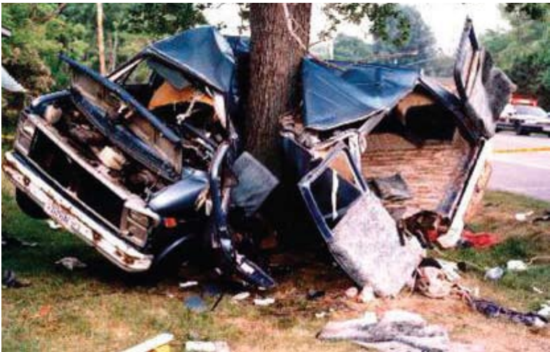
Roadside trees are fixed object hazards for vehicles leaving the traveled way.
