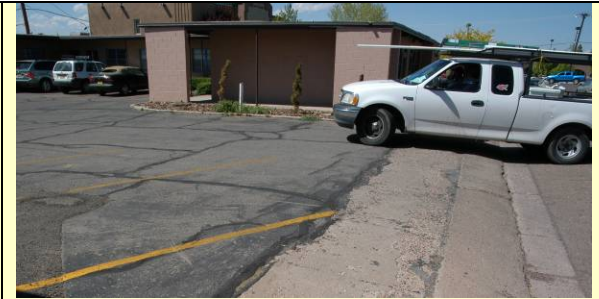
View of parking lot along Luisa Road. Photo shows where angle parking leads directly onto the sidewalk as vehicles back out of the space.
