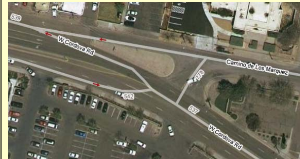
Aerial from Google Maps shows the skewed intersection of Cordova Road and Marquez where multiple access points create several conflicting movements.
