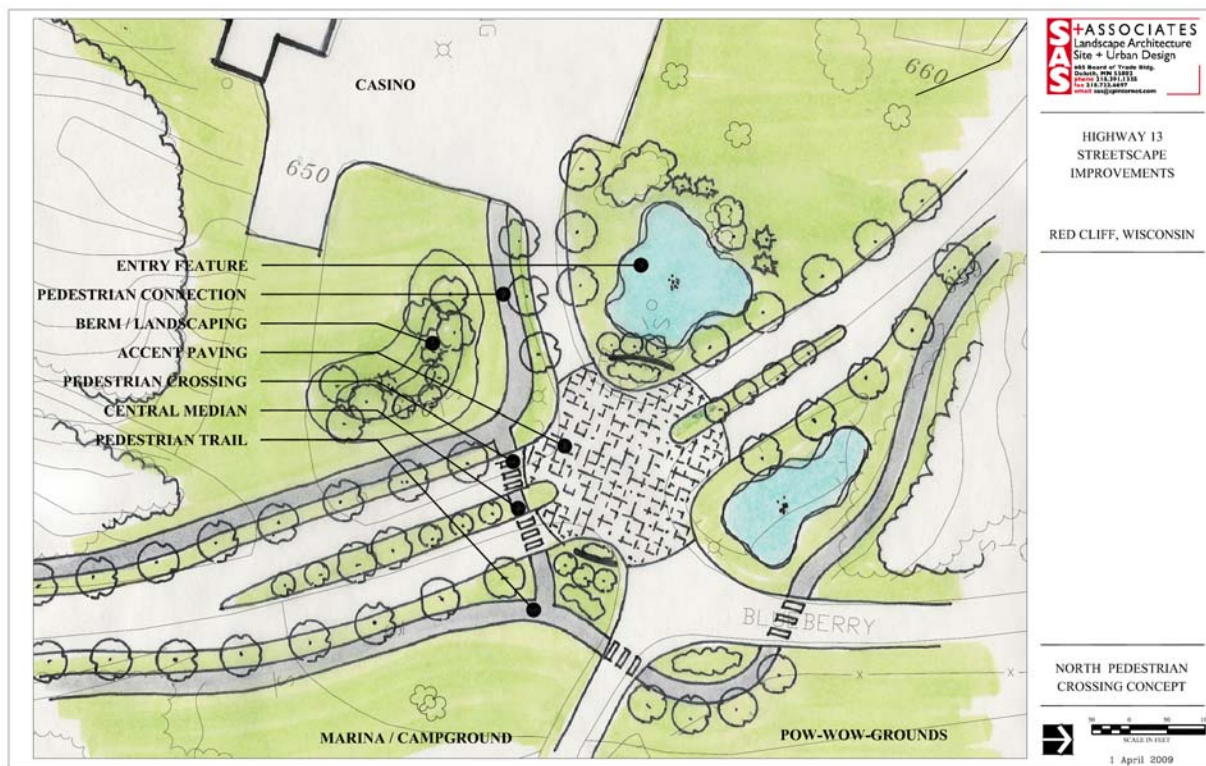
Figure 2. Conceptual Design for Highway 13 at Blueberry Rd.
