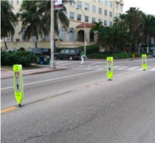
Figure 3.8 Picture of In-street “Yield to Pedestrians” Signs
