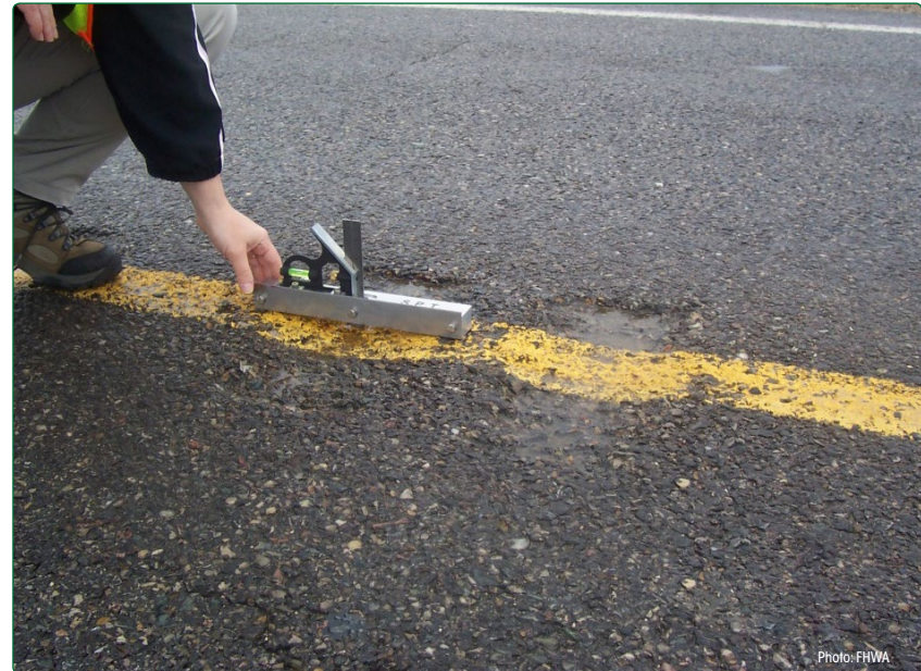
FIGURE 5. Measuring Milled Rumble Strips
