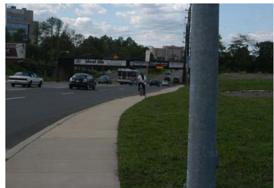
View of Route 70 just west of the railroad bridge. The bicyclist is biking on the sidewalk because of lack of a bikeable shoulder. The sidewalk is not wide enough to accommodate bicyclist and pedestrian traffic.
