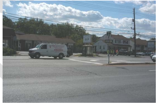
Photo of the intersection at Cornell Avenue, showing the current location of the eastbound bus stop on the southwest quadrant. The photo shows the absence of a crosswalk at this location, but also illustrates the potential impediments to installing a crosswalk (i.e., wide cross-section and limited median).
