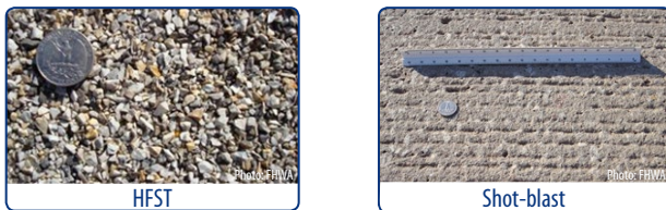
Figure 2. HFST Treatment Texture Compared to Shot-blasting Texture
