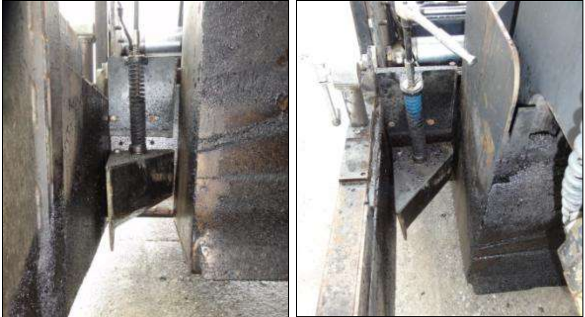
Figure 12. TransTech Shoulder Wedge Maker bolted to the paver screed.
