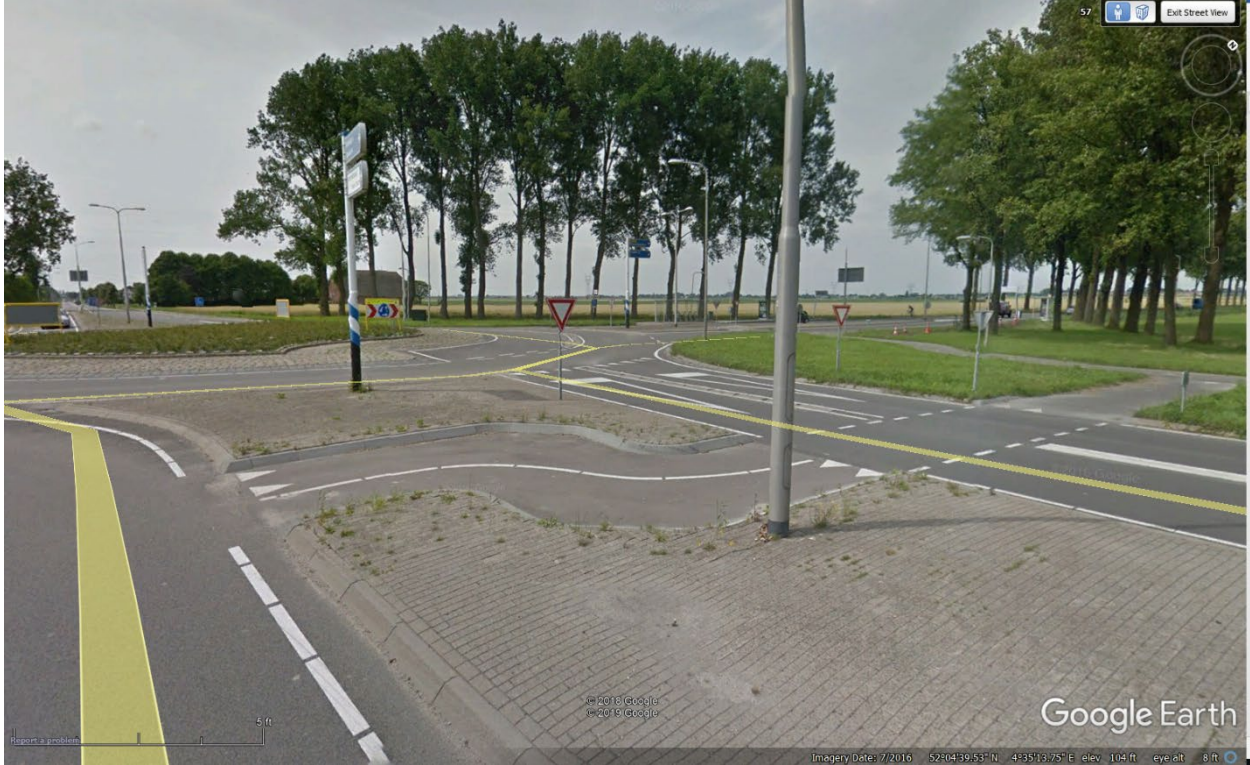
Figure 23. Photograph. Example of a chicane in a splitter island to encourage cyclists to perform a two-stage crossing.
