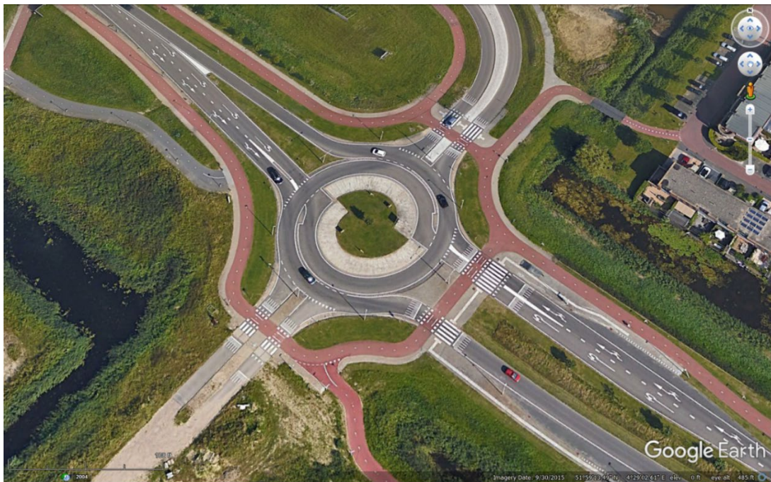
Figure 14. Photograph. New design for starting the inner lane used in the Netherlands.
