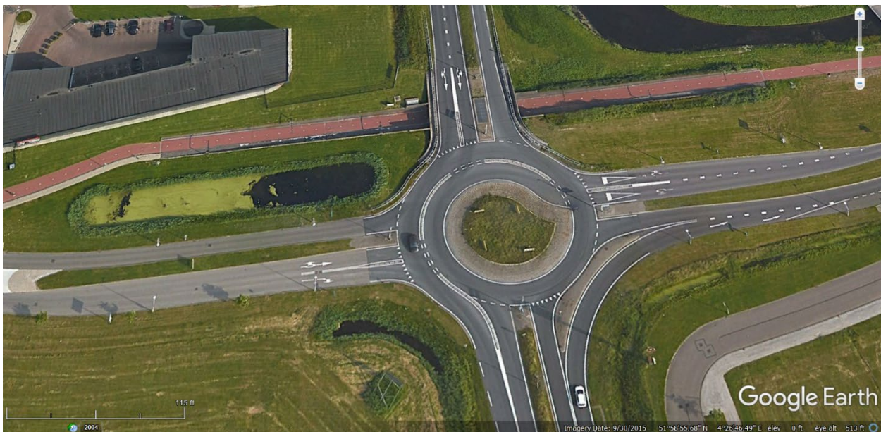
Figure 24. Photograph. Example of a grade separated bicycle facility at a turbo roundabout in South Holland.
