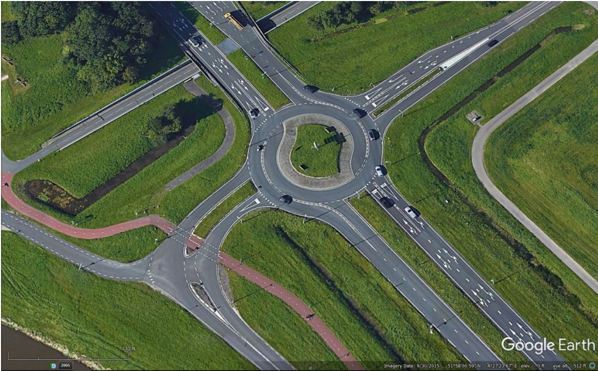
Figure 13. Photograph. Old design for starting the inner lane used in the Netherlands.
