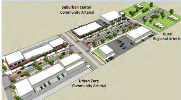
Figure 10. A rendering of roadway types as they differ from an Urban Core to Rural
