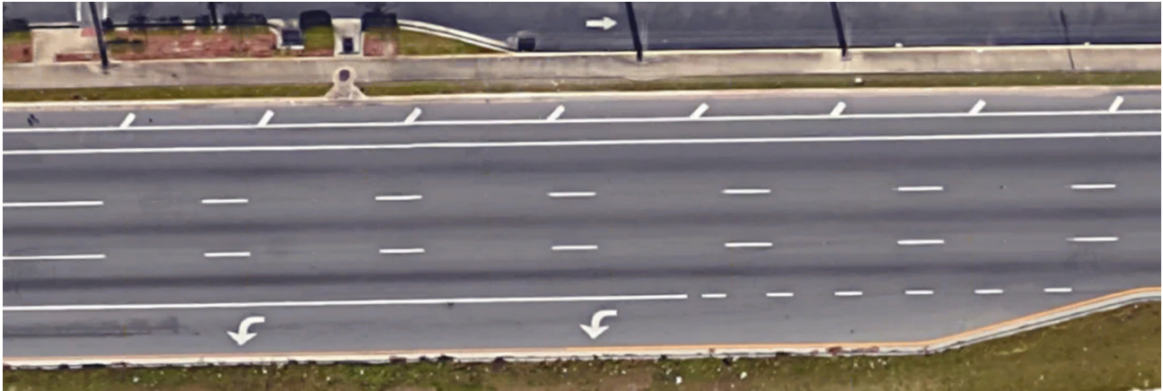
Figure 5. West Colonial Drive, east of the Pine Hills Road intersection, with a buffer between the bicycle lane and the curb (Map data: ©Google).
