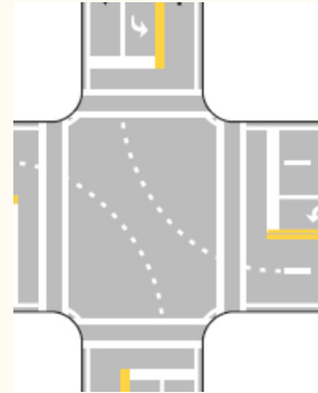
Example of dotted line markings to extend the left-turn lane line markings into the intersection (Source: MUTCD).
