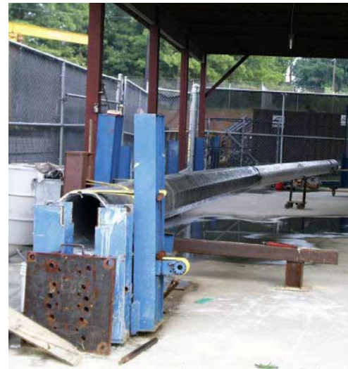
Figure 6. Photo. Composite utility pole undergoing strength testing. 23
