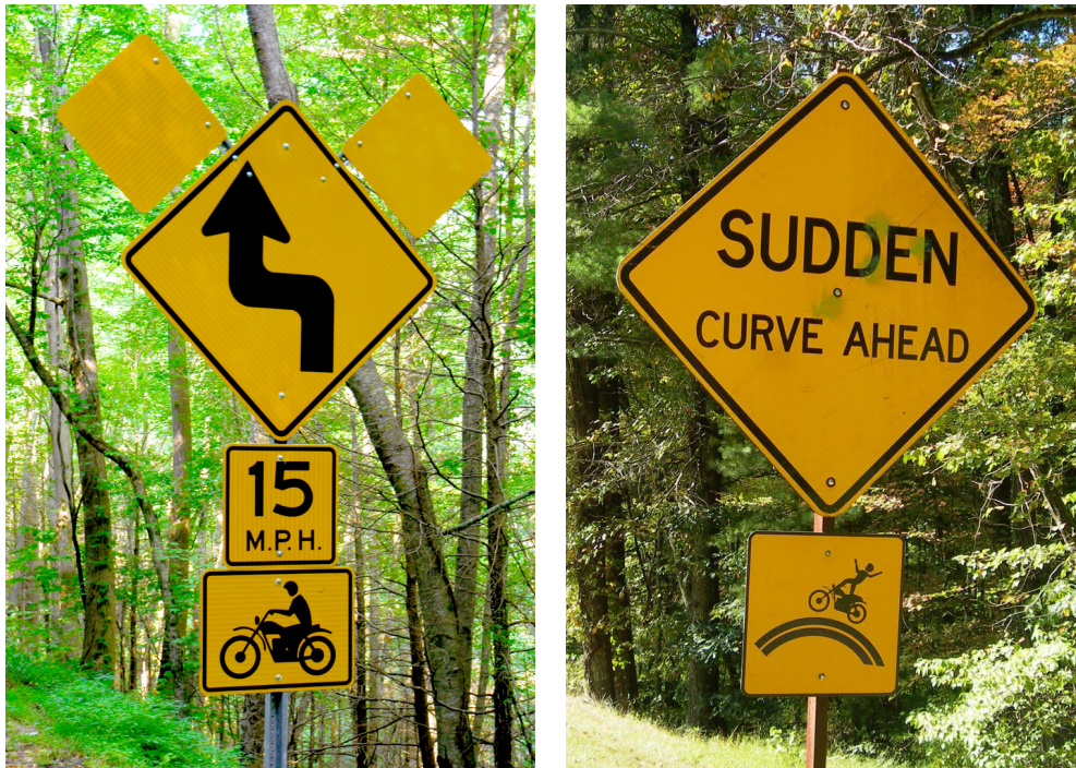
Left: NCDOT installed signage on North Carolina State Route 28 that includes curve warning signage, flagging, and a supplemental advisory speed plaque in addition to the motorcycle-specific supplemental plaque (Credit: Dan Nabors). Right: The “motorman” supplemental motorcycle plaque, which is not MUTCD-compliant, on the Blue Ridge Parkway (Credit: NPS).
