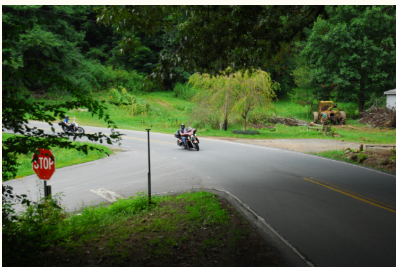
Photo showing motorcyclist crossing centerline on a sag vertical curve and horizontal curve. There is an intersecting roadway and driveway within the curve. (Credit: Dan Nabors)
