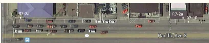
Top: Section of SR 7 near S 64th Street where the road transitions from a section with unmarked, on-street parking to a narrower section no on-street parking. The parking is not defined with an edgeline, creating a wide outside lane that may encourage unintended maneuvers and speeding. (Credit: Dan Nabors) Bottom: Example of pavement markings that could define on-street parking. The markings can be used to restrict parking near driveways and intersections, improve visibility of intersections, and define parking so that there is a consistent cross-section throughout the corridor. Signage can be used to restrict parking during times of day when crashes are more prevalent (e.g., 2 PM to 7 PM). (Source: Google Maps)
