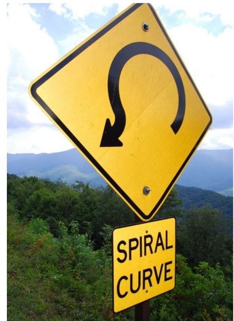
A Spiral Curve Warning Sign. Note: sign not MUTCD-compliant. (Credit: Dan Nabors)
