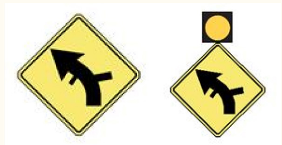
Examples of intersection warning signs that depict the location of intersections along a curve. The sign on the left is an example of sign that could be used for northbound drivers on SR 7, as it depicts the intersection with Alder Cutoff Road on the right, and the parking lot entrance on the left. Consider combining the warning sign with a flashing beacon, as shown.
