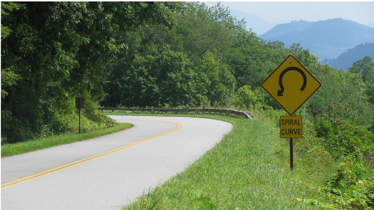
Spiral Curve Warning Sign along the Blue Ridge Parkway. (Credit: Dan Nabors)
