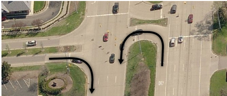
Exhibit 4-8. Example of U-turn/right-turn conflict. (3)
