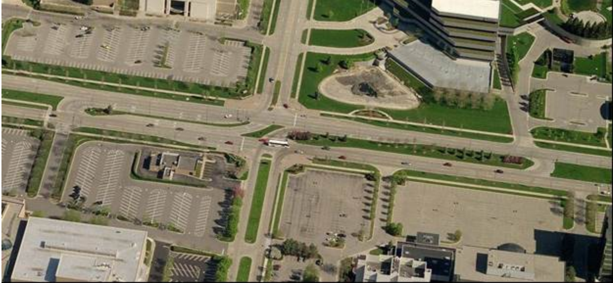
Exhibit 7-7. Signalized RCUT intersection on Big Beaver Road in Troy, MI with six-lane major street and four-lane minor street. (3)
