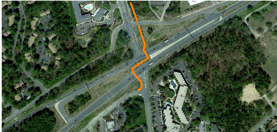
Exhibit 3-9. Median shared-use path design for the US Route 15/501 RCUT intersection in North Carolina. (25)
