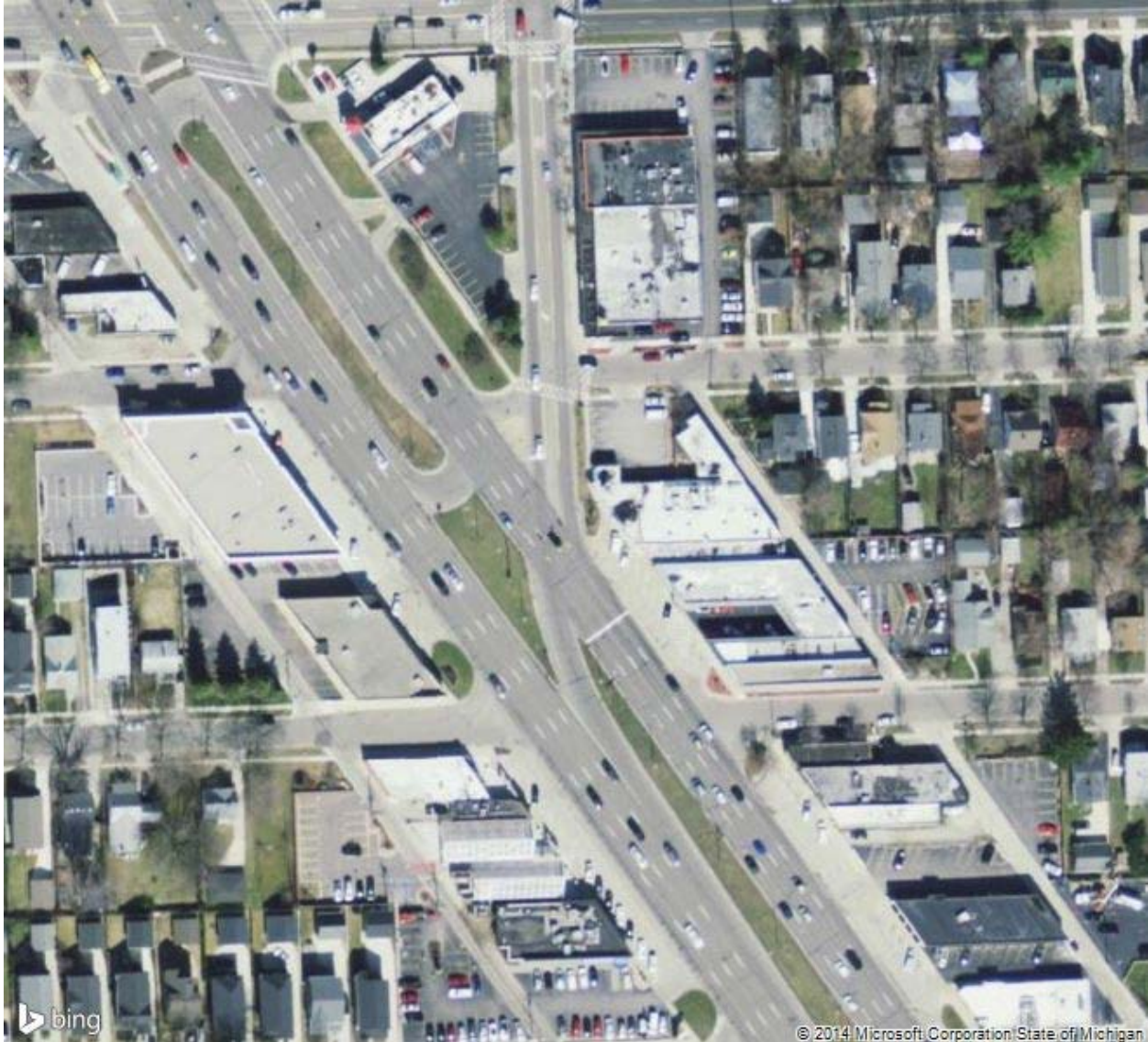
Exhibit 7-11. Minor street left turn crossover with a merge on Woodward Avenue in Birmingham, MI. (2)
