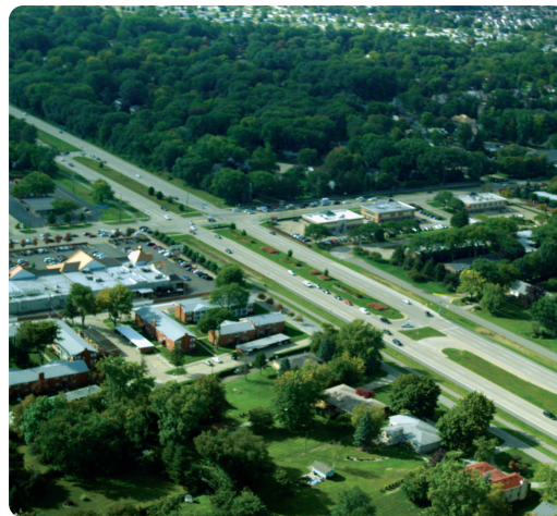
MUT Intersection, Metropolitan Parkway, Clinton Township, MI Source: MUT Case Study Video FHWA-SA-14-053
