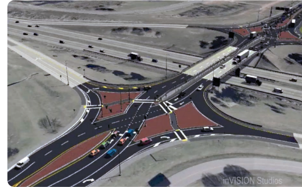
Computer Simulation of the Proposed Interchange Source: DDI Case Study Video FHWA-SA-14-047
