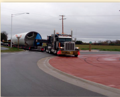
Figure 1: Oversize truck entering a roundabout designed to accommodate OSOW vehicles.
