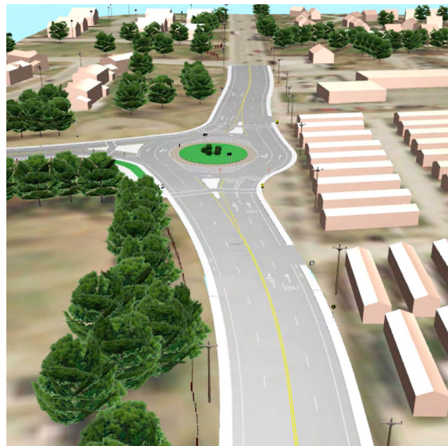
Figure 7: Images from both 3-D models comparing the signalized intersection and roundabout alternatives at Coddington Highway and the proposed connector road (Burma Road South)
