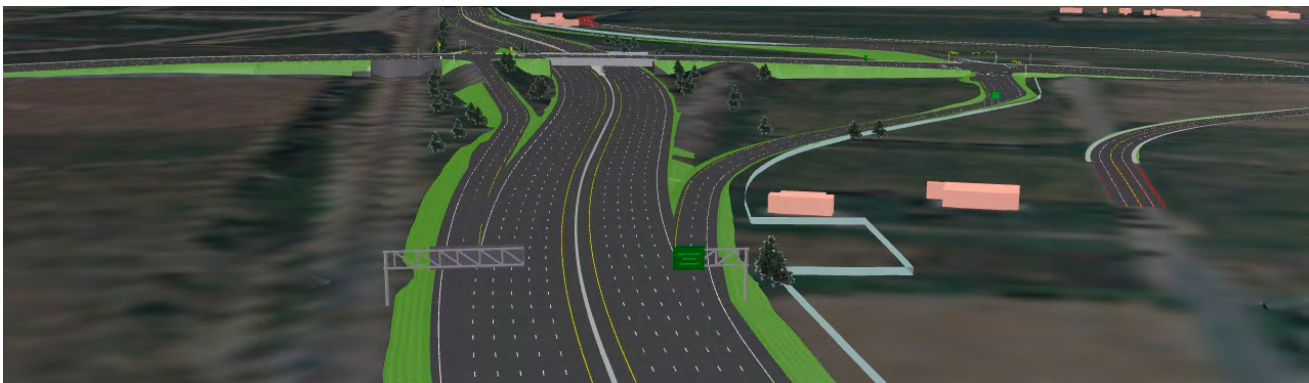
Figure 39: Image from 3-D model showing closeness of interchange ramps and multilane cross section
