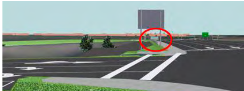
Figure 38: Image from 3-D model showing potential for overpass structure to obstruct sight distance of drivers at SB exit ramp
